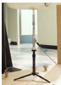
Figure 7.1 Dipole Validation Test Setup
