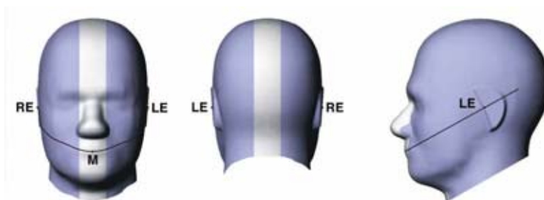
Figure 5.1 Front, back and side view of SAM
