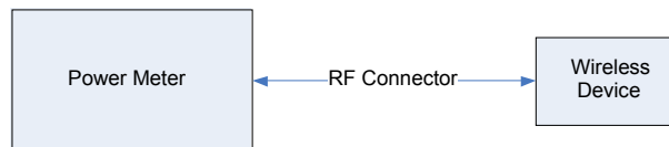
Figure 11-2 Power Measurement Setup
