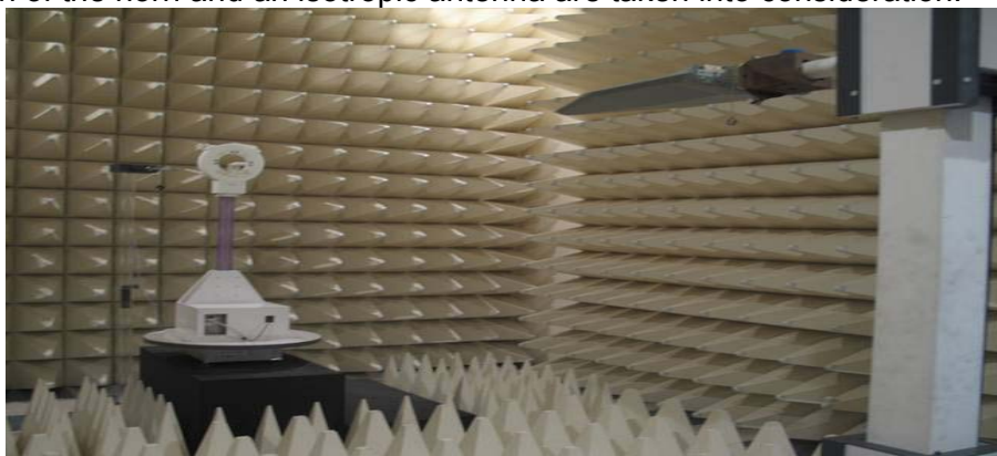
Figure2. Photograph of 3m Fully-Anechoic Chamber
