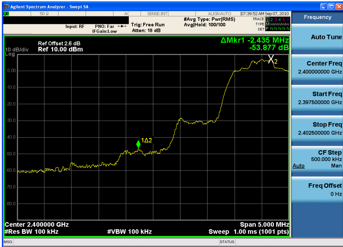
Plot 6-6. Band Edge Plot (Bluetooth (EDR) – Ch. 0)
