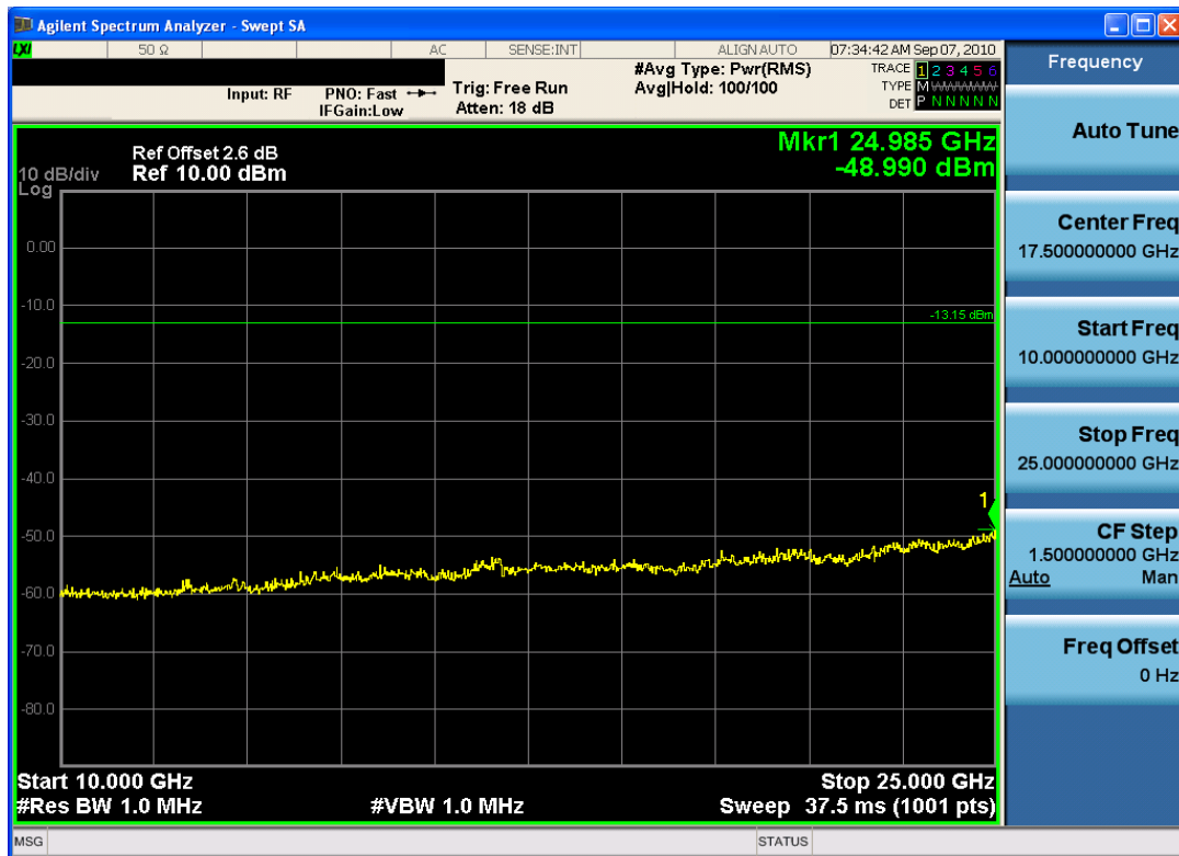
Plot 6-17. Conducted Spurious Plot (Bluetooth – Ch. 78)
