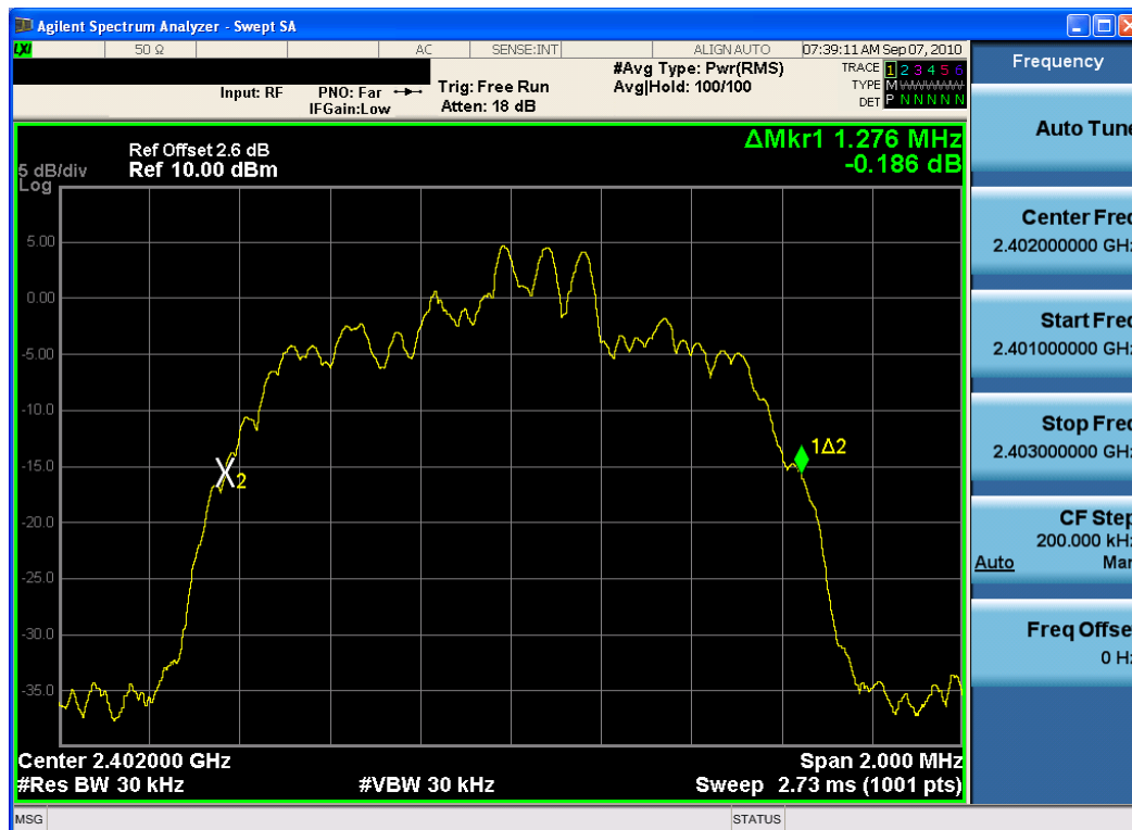
Plot 6-1. 20dB Bandwidth Plot (Bluetooth (EDR) – Ch. 0)
