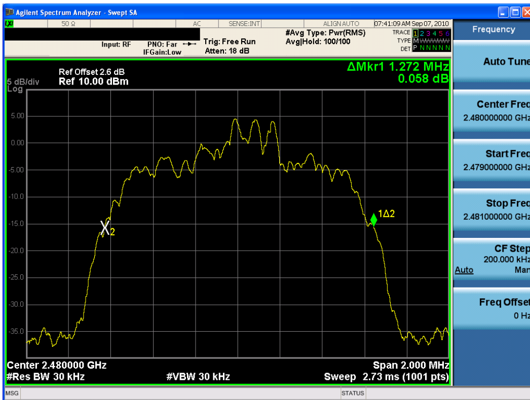
Plot 6-3. 20dB Bandwidth Plot (Bluetooth (EDR) - Ch. 78)
