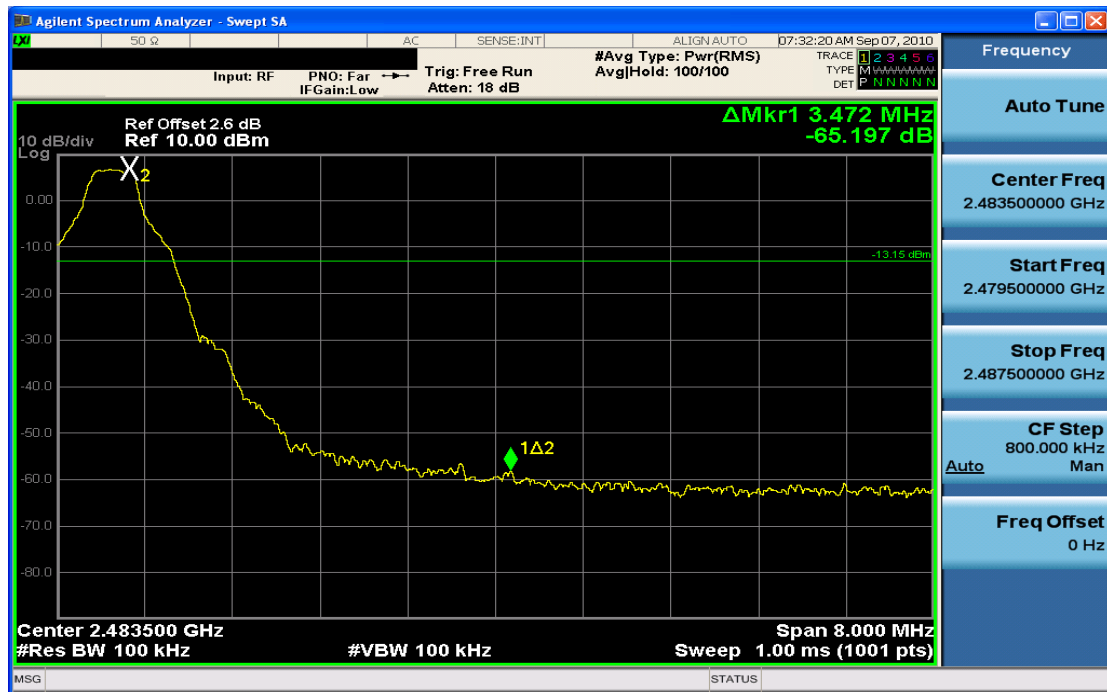
Plot 6-5. Band Edge Plot (Bluetooth – Ch. 78)
