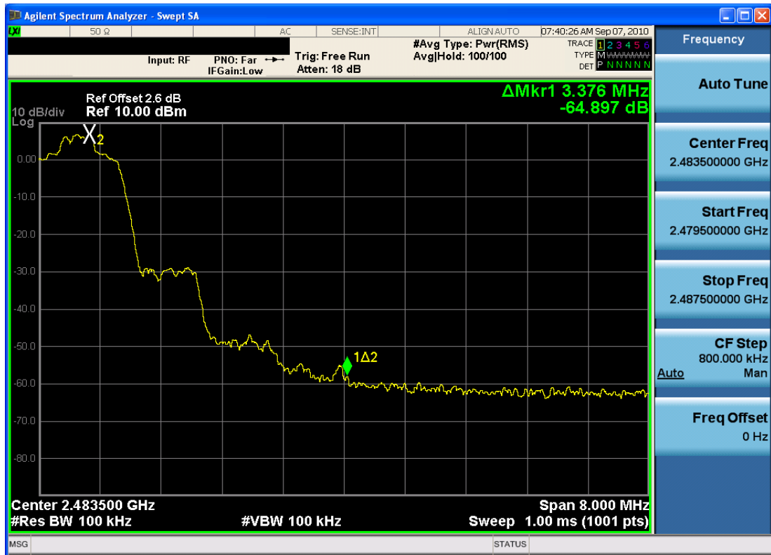
Plot 6-7. Band Edge Plot (Bluetooth (EDR) – Ch. 78)
