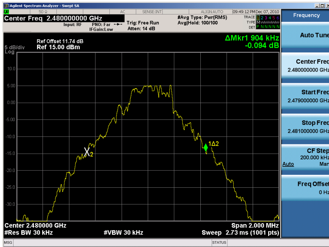
Plot 6-3. 20dB Bandwidth Plot (Bluetooth, 1Mbps – Ch. 78)
