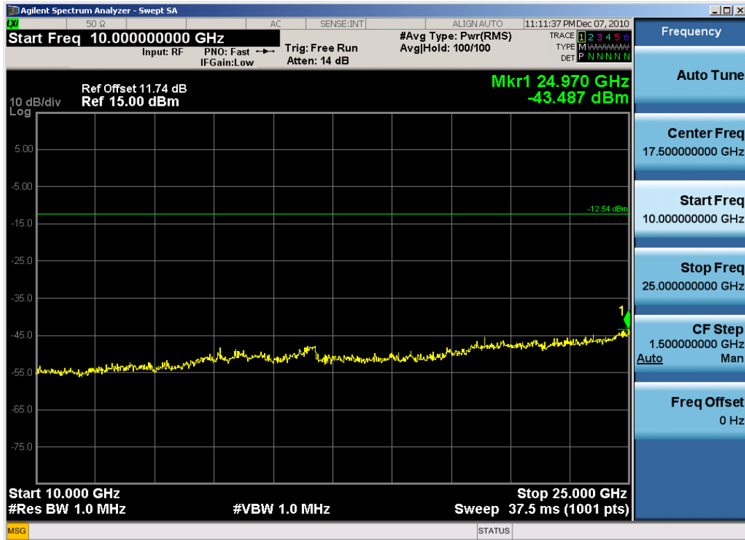
Plot 6-23. Conducted Spurious Plot (Bluetooth, 3Mbps – Ch. 78)
