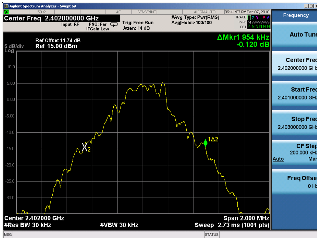
Plot 6-1. 20dB Bandwidth Plot (Bluetooth, 1Mbps – Ch. 0)
