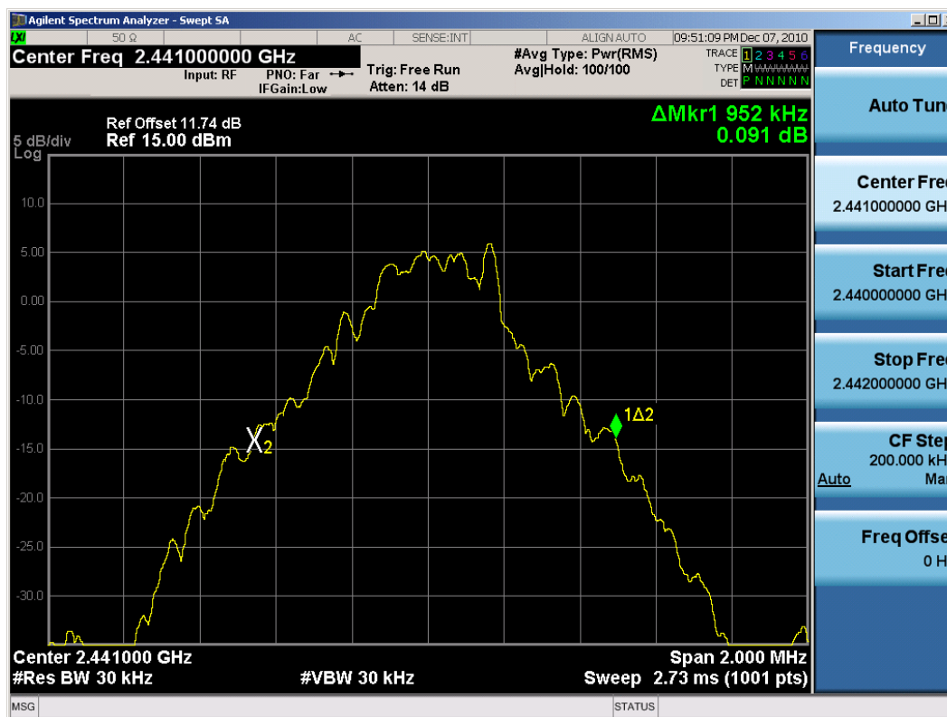
Plot 6-2. 20dB Bandwidth Plot (Bluetooth, 1Mbps – Ch. 39)
