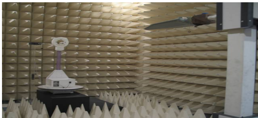
Figure2. Photograph of 3m Fully-Anechoic Chamber
