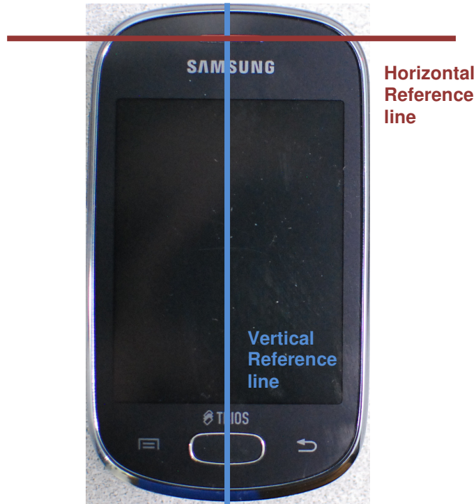
SAR Test Setup Photo 11: DUT Reference Lines
