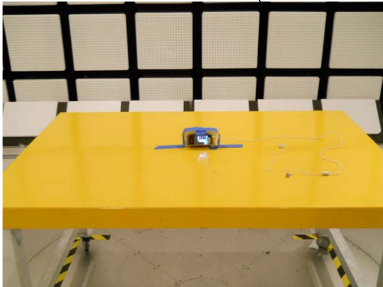
Y-AXIS FRONT + HEADSET PHOTO (worst-case orientation)
