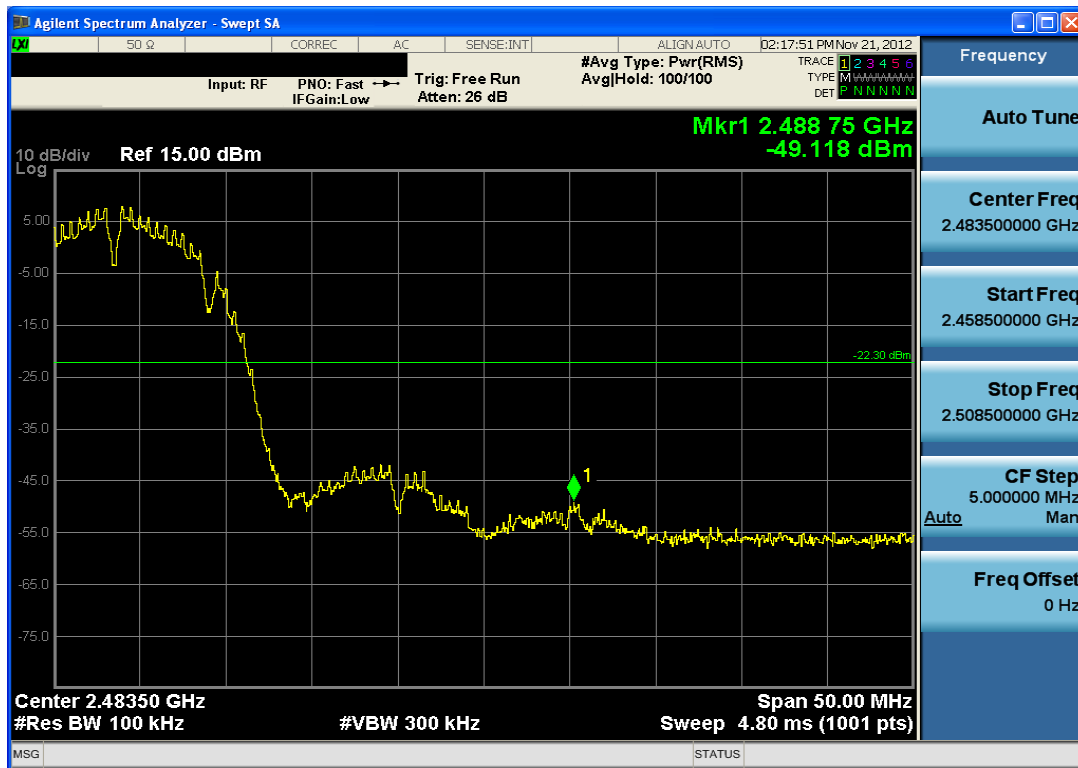
Plot 6-20. Band Edge Plot (802.11b – Ch. 11)
