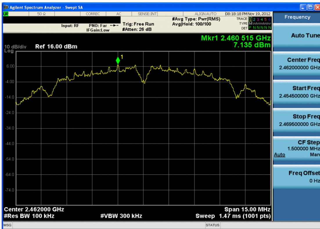
Plot 6-12. Power Spectral Density Plot (802.11b – Ch. 11)
