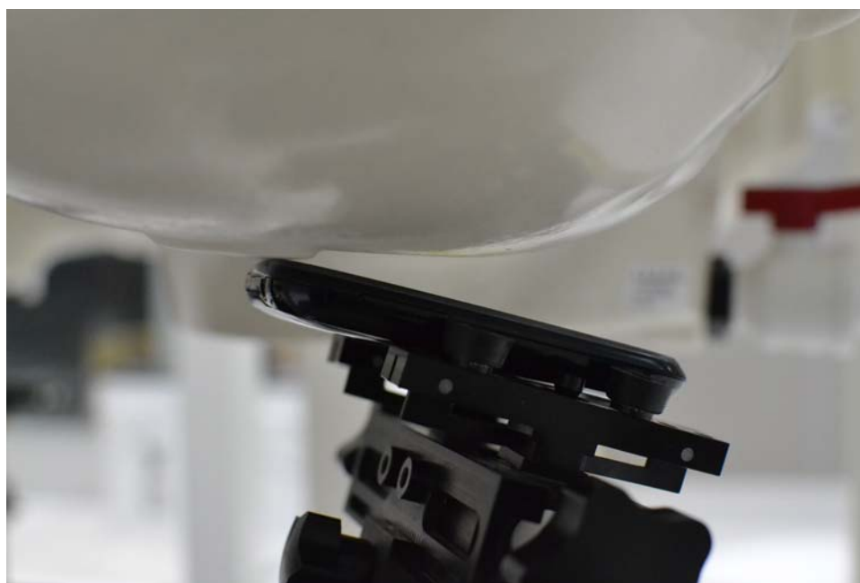
SAR Test Setup Photo 2 - Right Tilt
