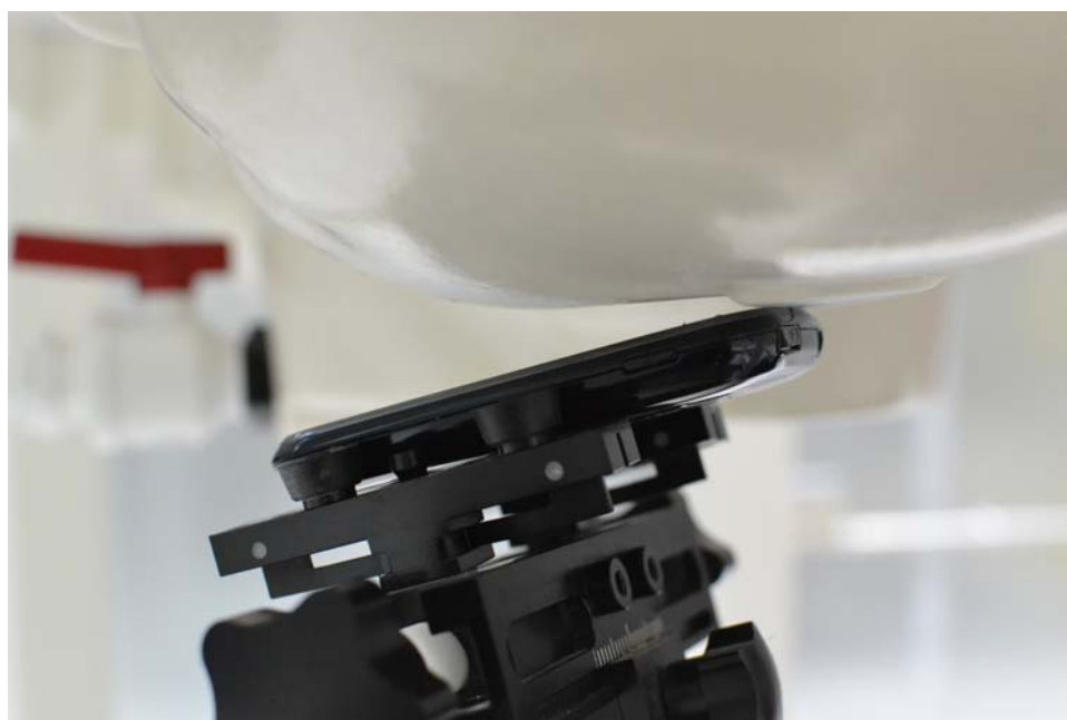
SAR Test Setup Photo 4 - Left Tilt
