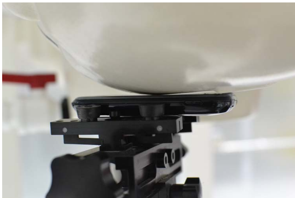
SAR Test Setup Photo 3 - Left Cheek
