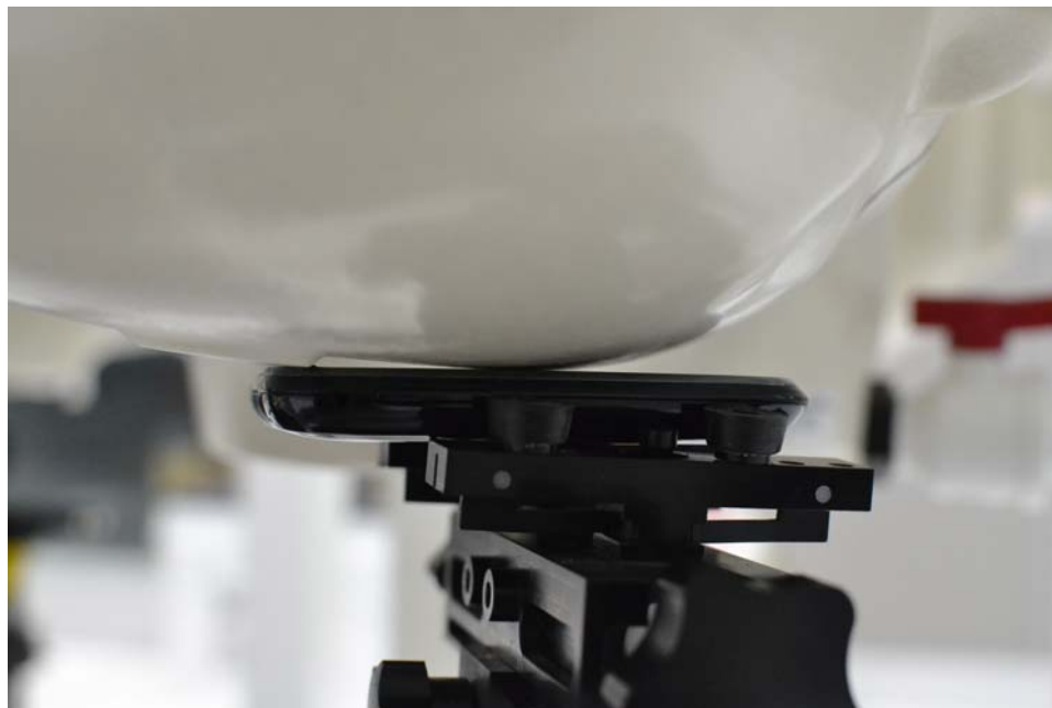
SAR Test Setup Photo 1 - Right Cheek
