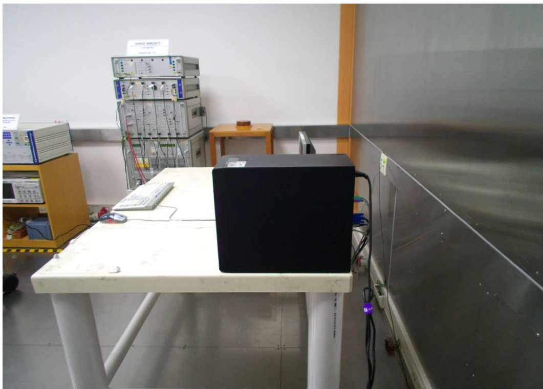
[ Conducted Disturbance – Rear ]
