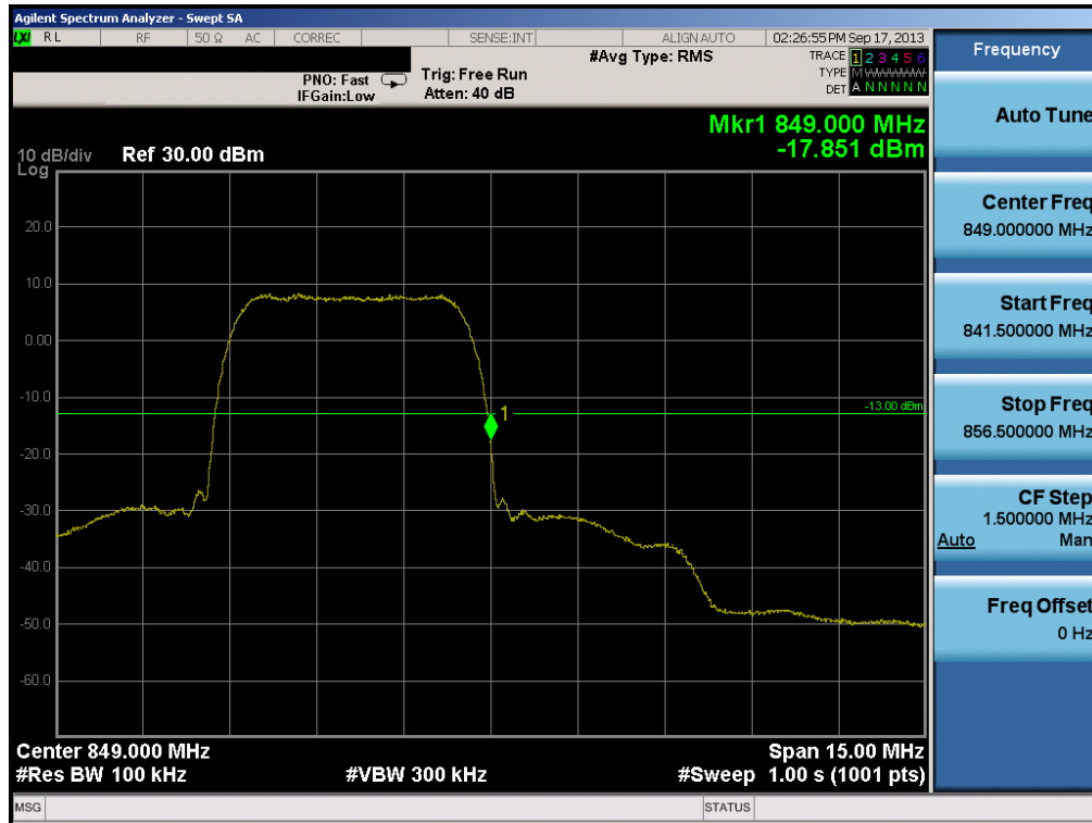
Plot 6-30. Band Edge Plot (Cellular WCDMA Mode – Ch. 4233)
