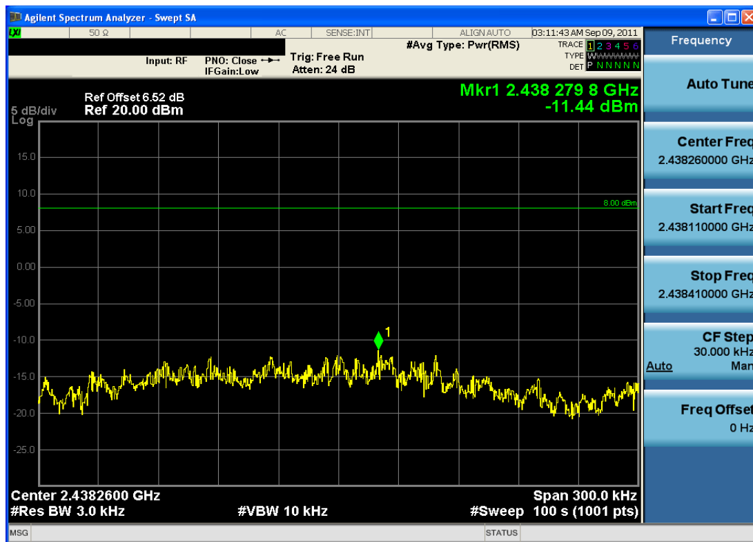
Plot 6-14. Power Spectral Density Plot (802.11g - Ch. 6)
