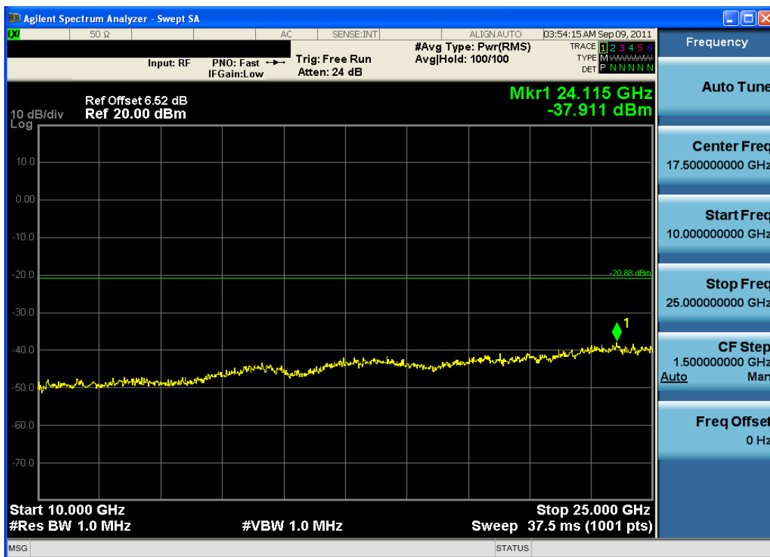
Plot 6-26. Conducted Spurious Plot (802.11b – Ch. 1)
