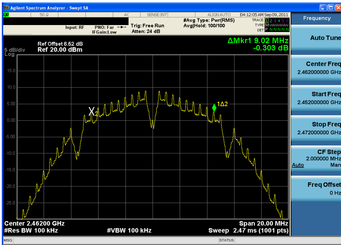
Plot 6-3. 6dB Bandwidth Plot (802.11b – Ch. 11)
