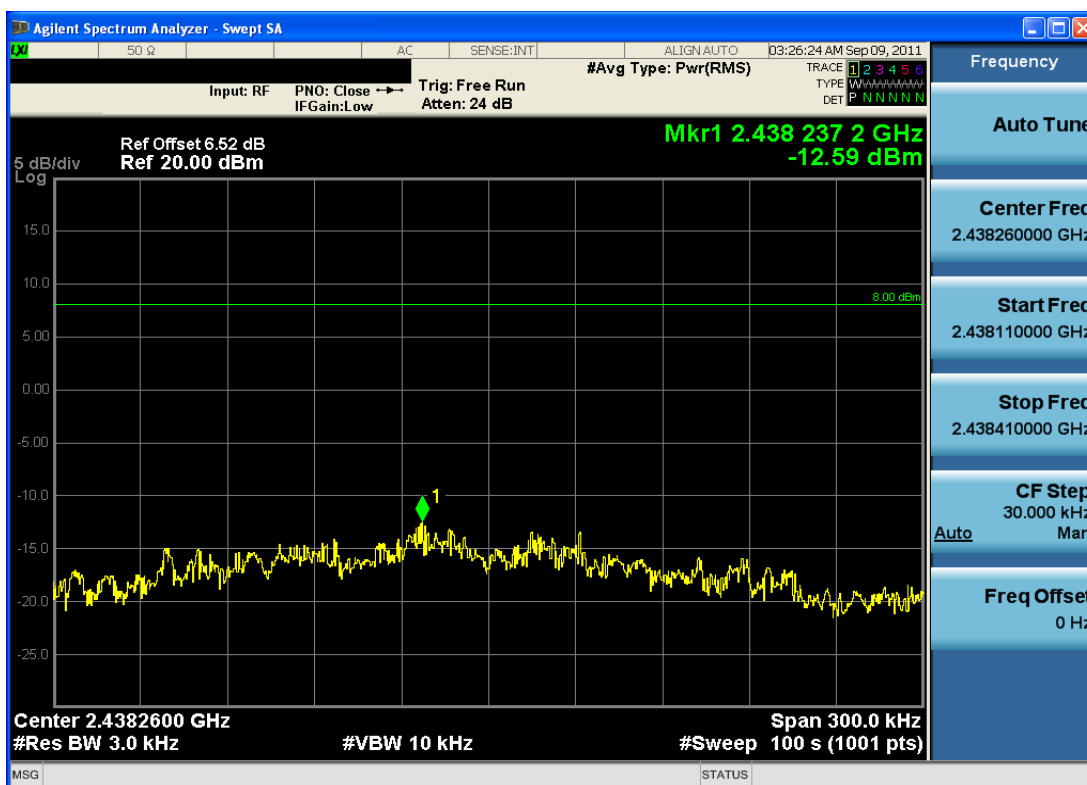
Plot 6-17. Power Spectral Density Plot (802.11n – Ch. 6)
