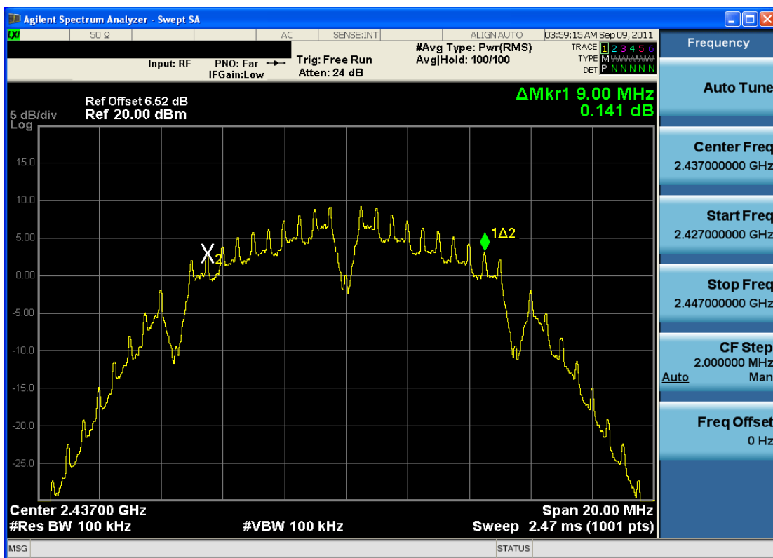
Plot 6-2. 6dB Bandwidth Plot (802.11b – Ch. 6)
