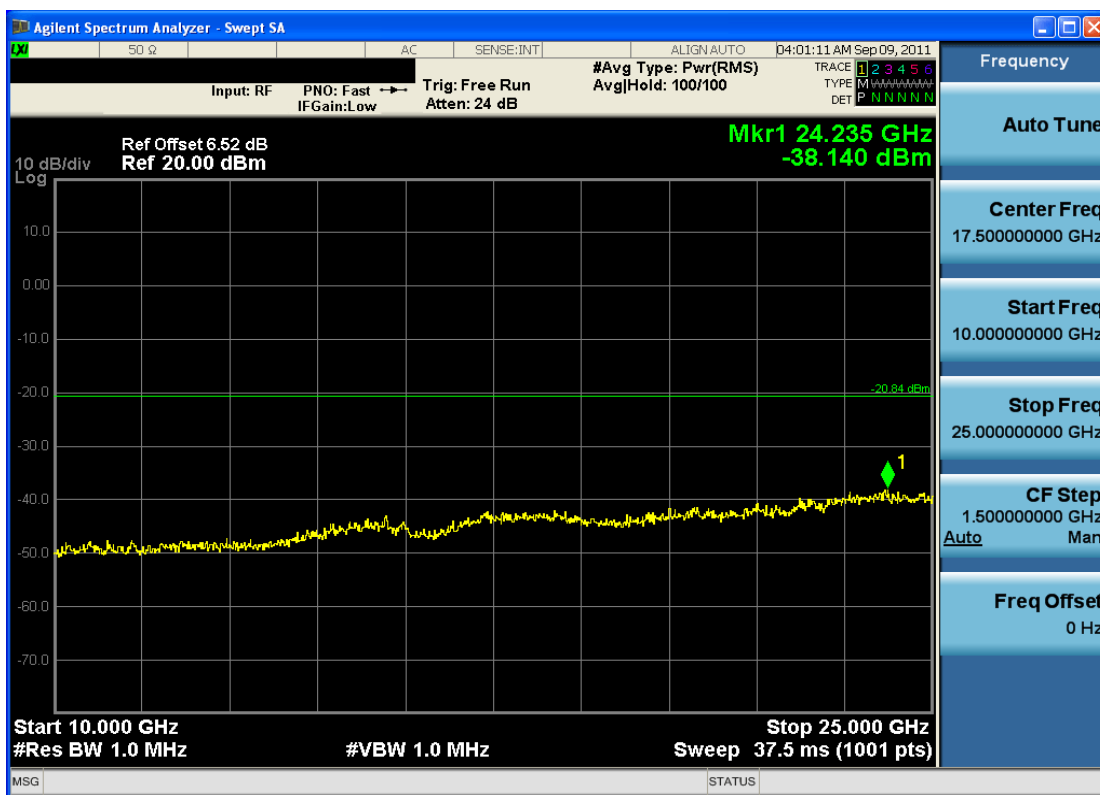
Plot 6-28. Conducted Spurious Plot (802.11b – Ch. 6)
