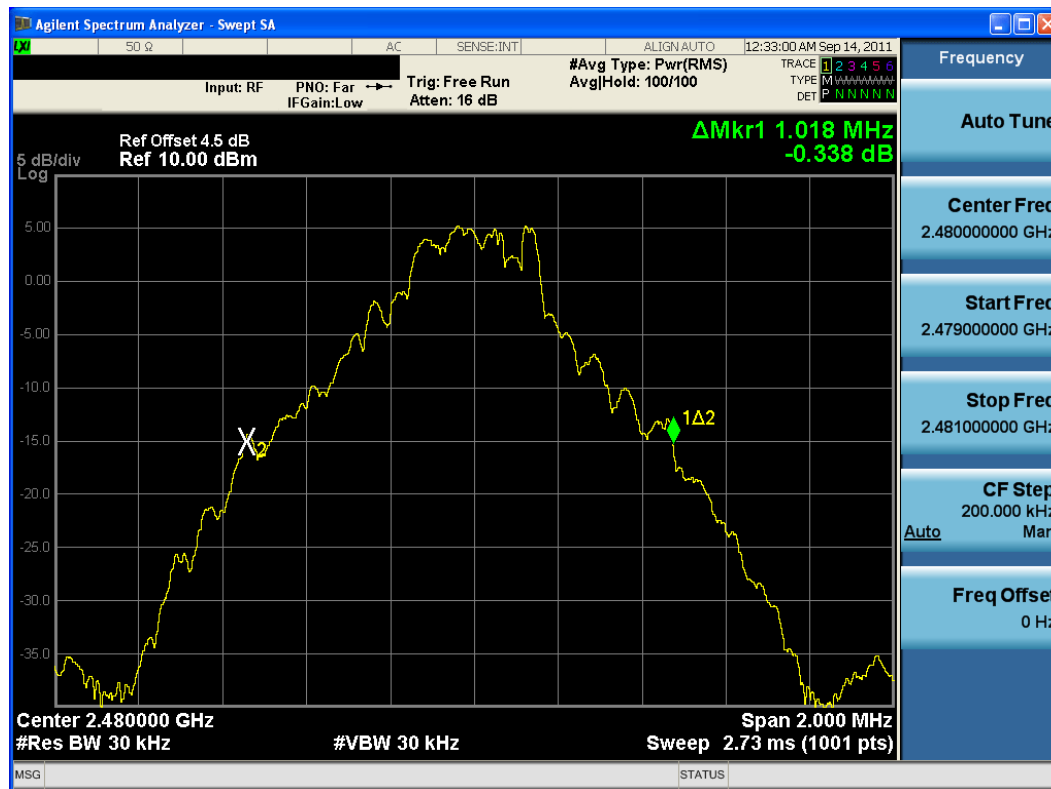
Plot 6-3. 20dB Bandwidth Plot (Bluetooth, 1Mbps – Ch. 78)
