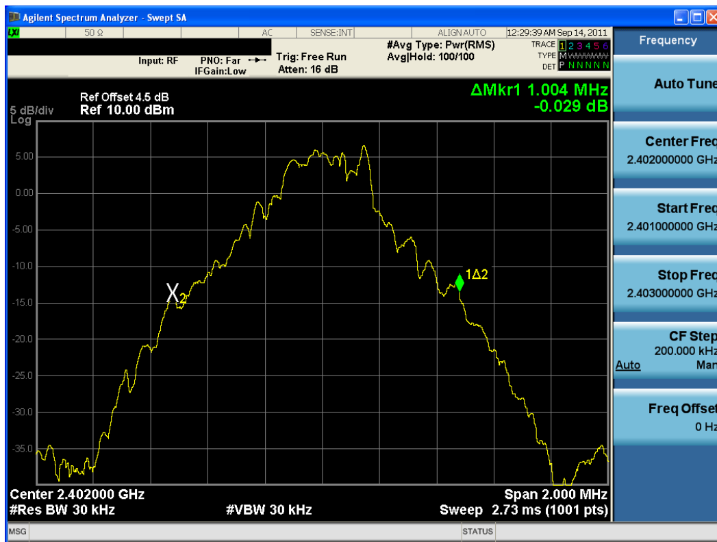
Plot 6-1. 20dB Bandwidth Plot (Bluetooth, 1Mbps – Ch. 0)
