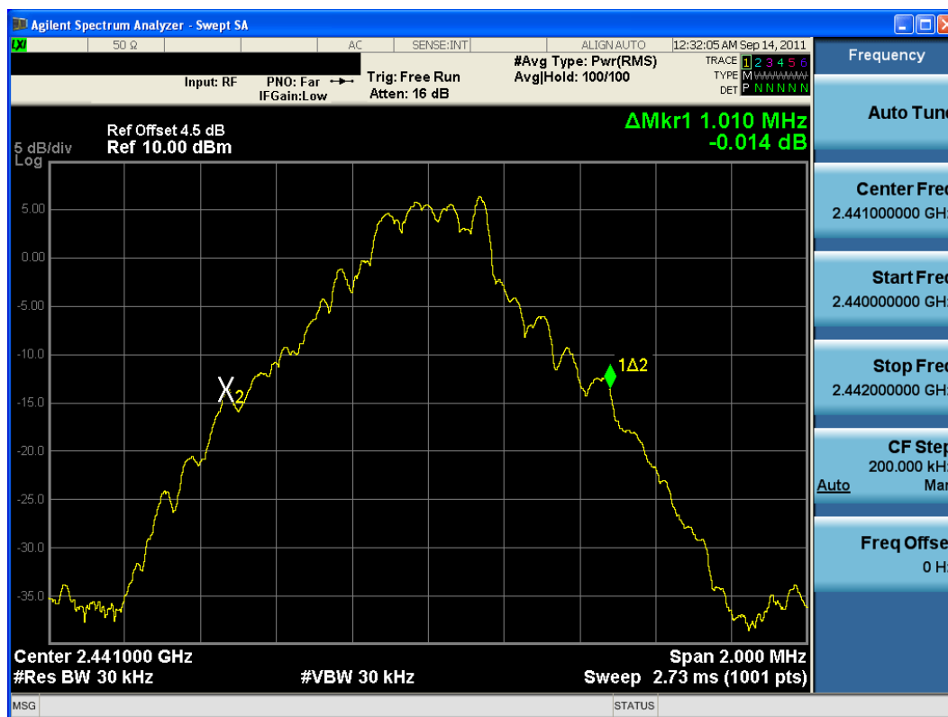
Plot 6-2. 20dB Bandwidth Plot (Bluetooth, 1Mbps – Ch. 39)
