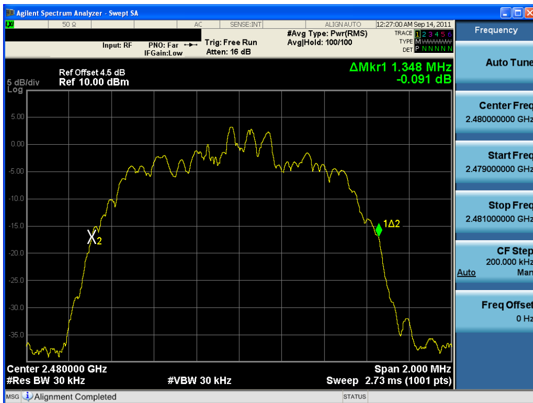
Plot 6-6. 20dB Bandwidth Plot (Bluetooth, 2Mbps – Ch. 78)
