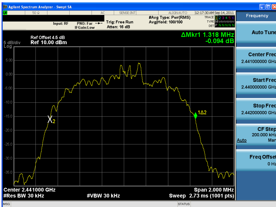
Plot 6-8. 20dB Bandwidth Plot (Bluetooth, 3Mbps – Ch. 39)
