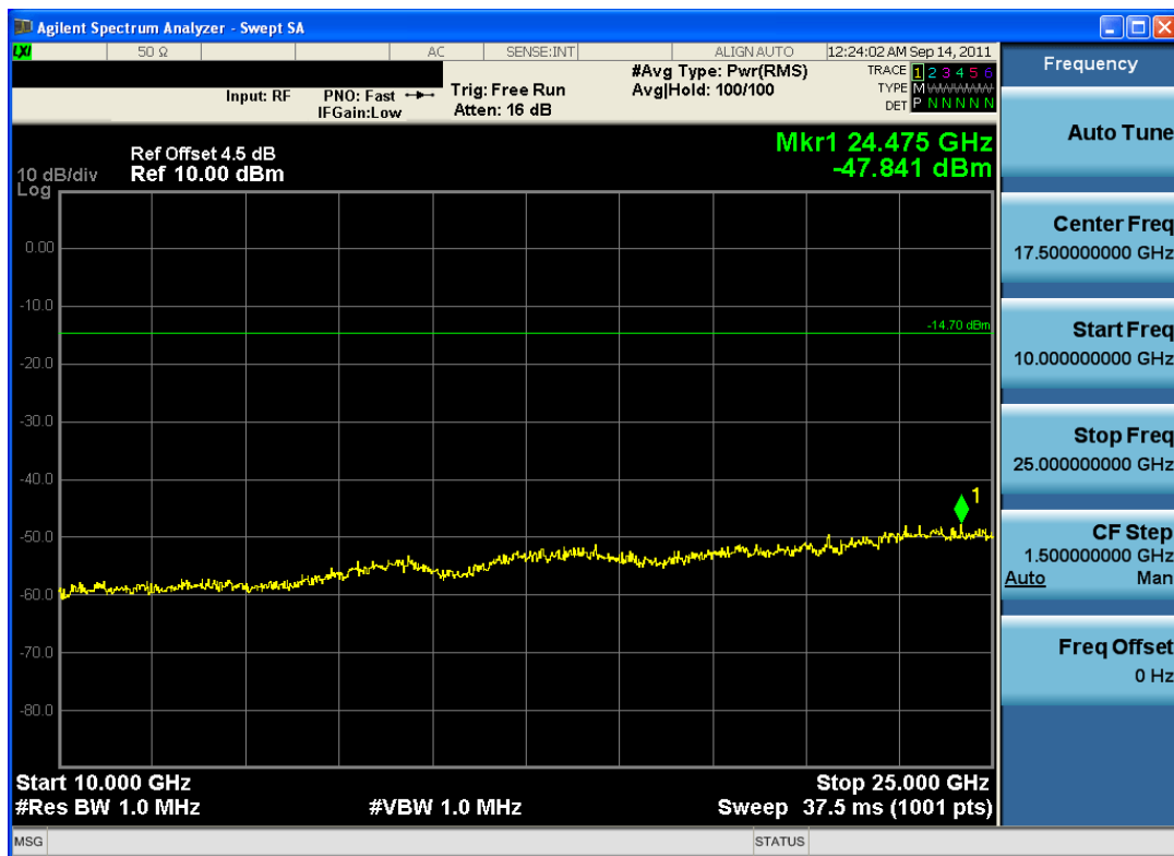
Plot 6-21. Conducted Spurious Plot (Bluetooth, 3Mbps – Ch. 78)
