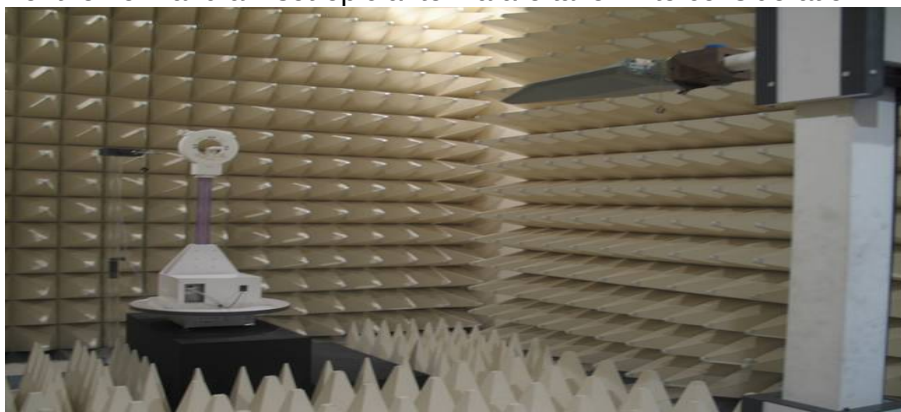
Figure2. Photograph of 3m Fully-Anechoic Chamber
