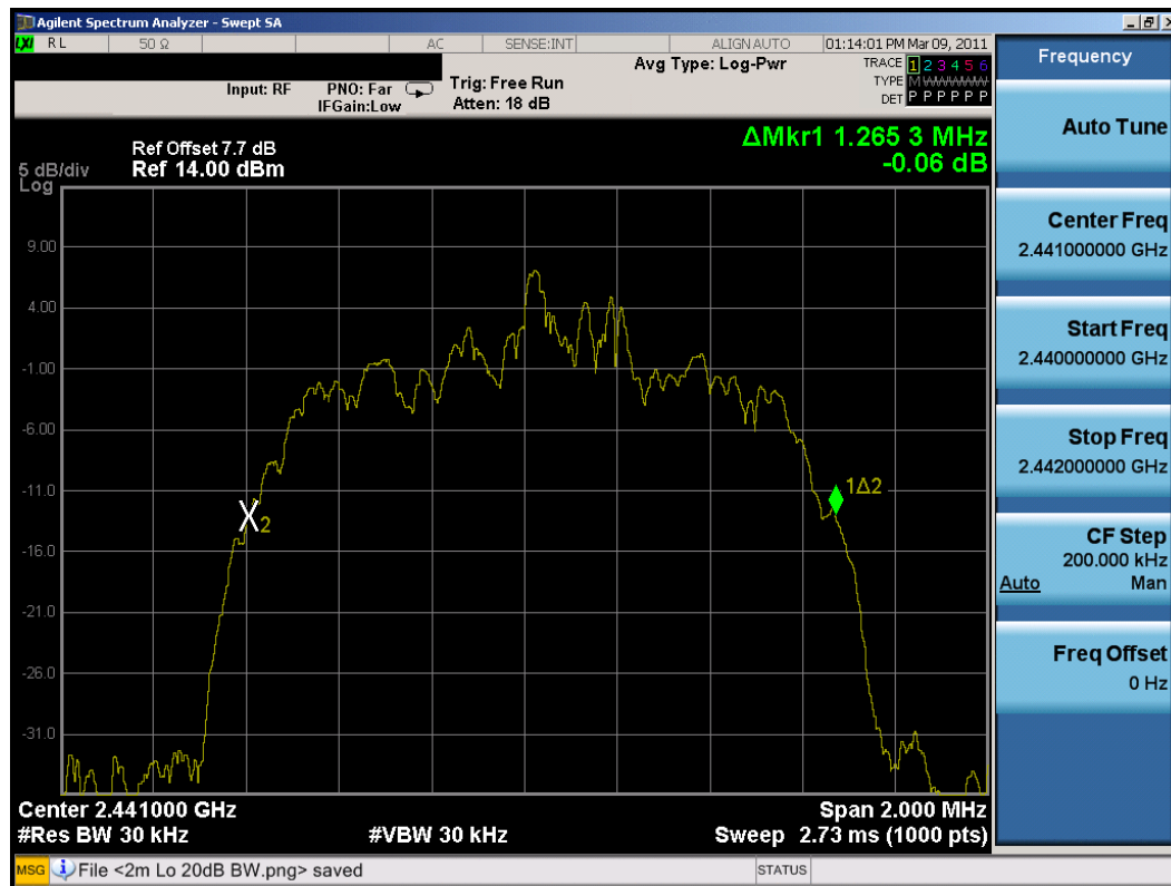
Plot 6-5. 20dB Bandwidth Plot (Bluetooth, 2Mbps – Ch. 39)
