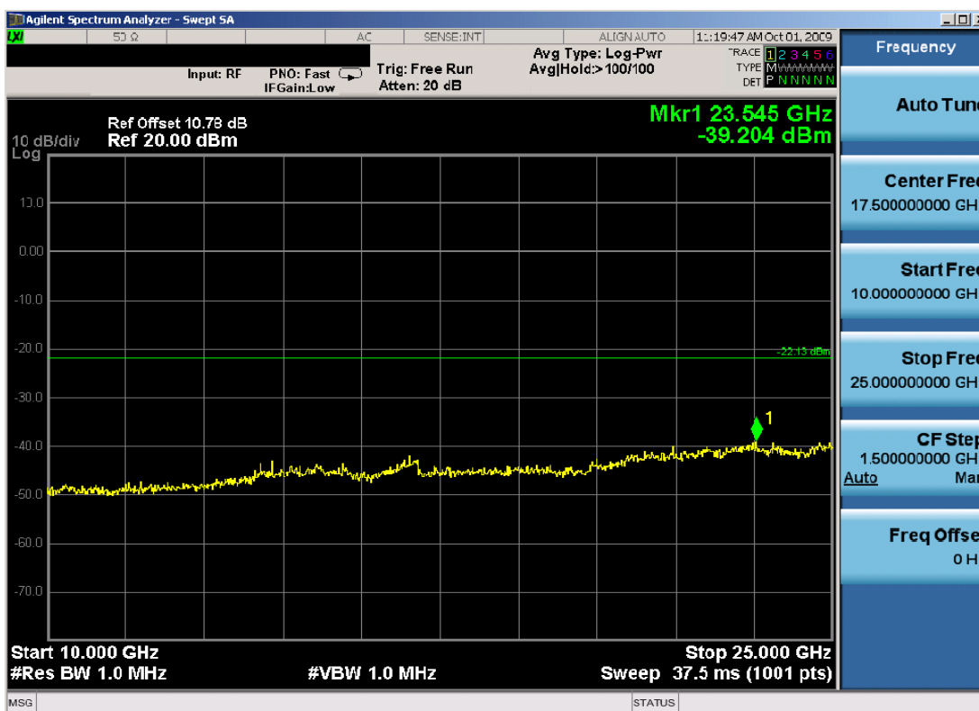
Plot 6-22. Conducted Spurious Plot (802.11b - Ch. 11)
