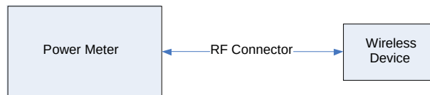
Figure 11-1 Power Measurement Setup
