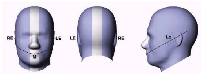
Figure 7-4 Front, back and side view of SAM Twin Phantom
