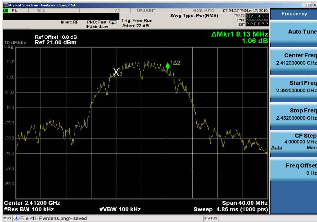
Plot 6-1. 6dB Bandwidth Plot (802.11b – Ch. 1)
