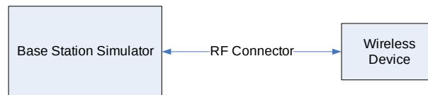
Figure 11-1 Power Measurement Setup
