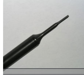
Figure 3.4 Probe Thick-Film Technique
