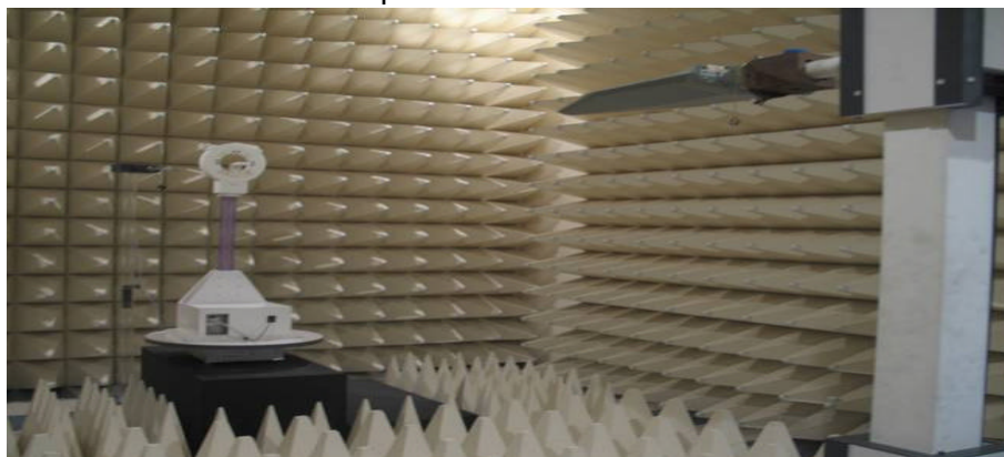
Figure2. Photograph of 3m Fully-Anechoic Chamber
