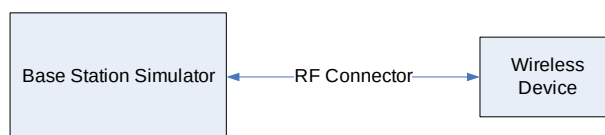
Figure 11-1 Power Measurement Setup
