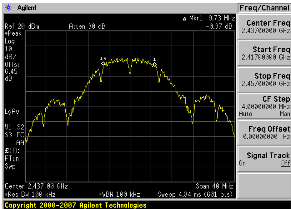
Plot 6-2. 6dB Bandwidth Plot (802.11b – Ch. 6)
