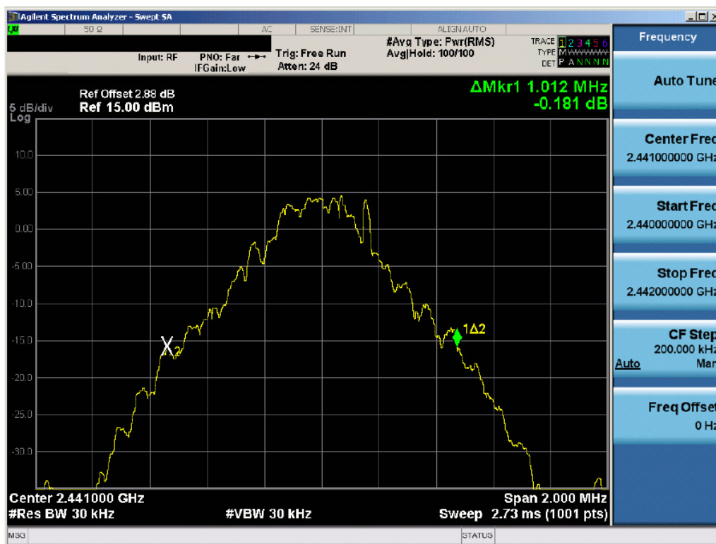
Plot 6-2. 20dB Bandwidth Plot (Bluetooth, 1Mbps – Ch. 39)
