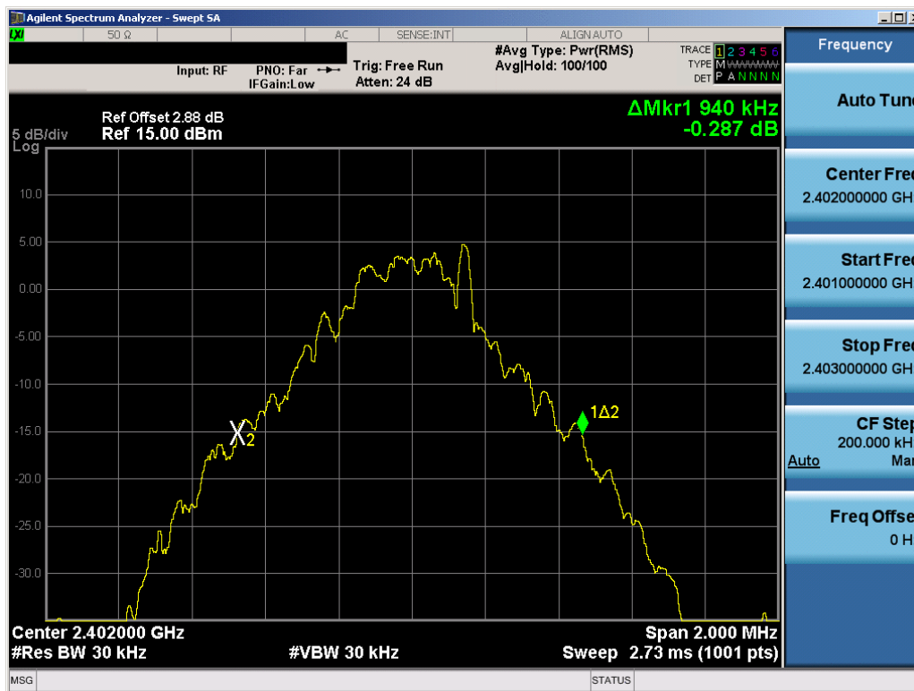
Plot 6-1. 20dB Bandwidth Plot (Bluetooth, 1Mbps – Ch. 0)
