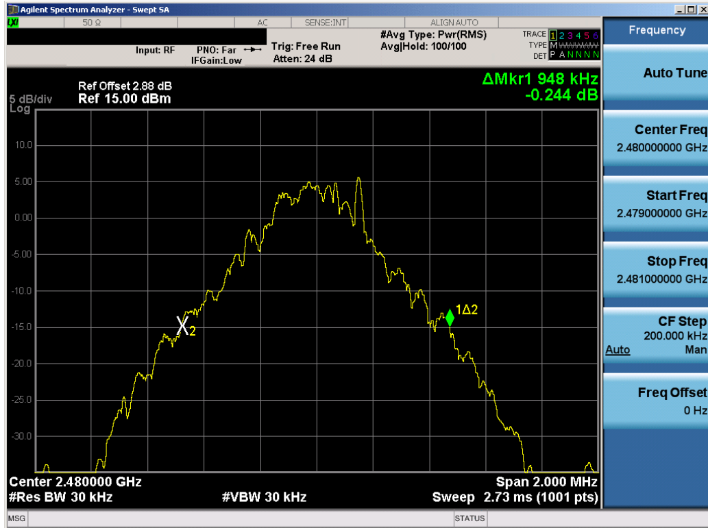
Plot 6-3. 20dB Bandwidth Plot (Bluetooth, 1Mbps – Ch. 78)
