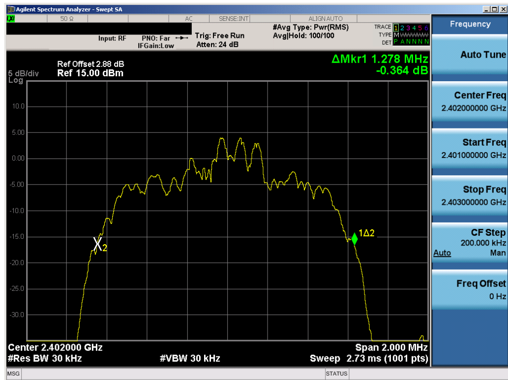
Plot 6-4. 20dB Bandwidth Plot (Bluetooth, 2Mbps – Ch. 0)
