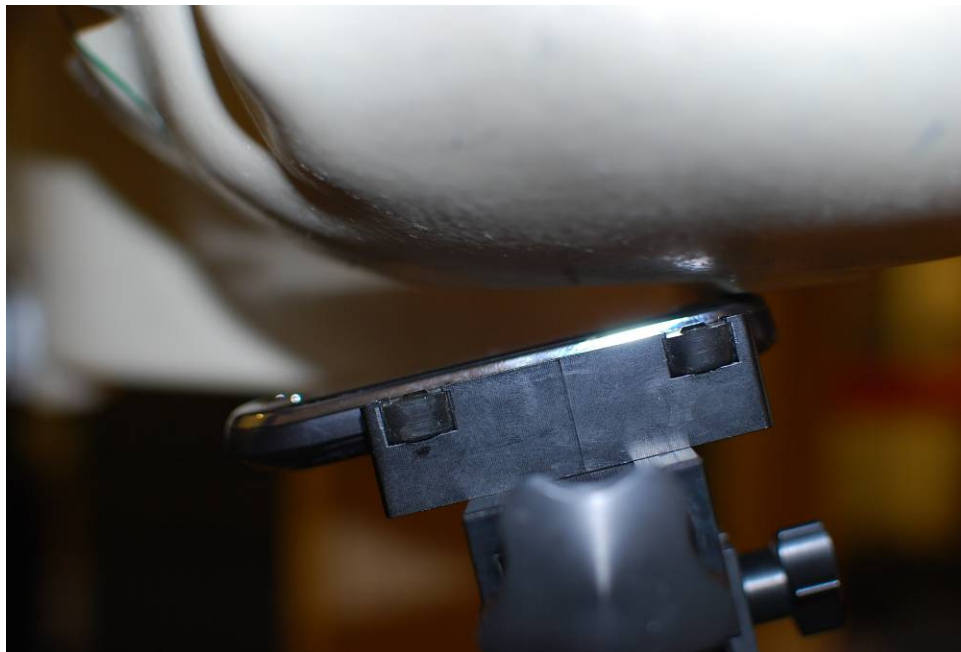
Figure 21-4 SAR Test Setup Photo 4 Left Tilt
