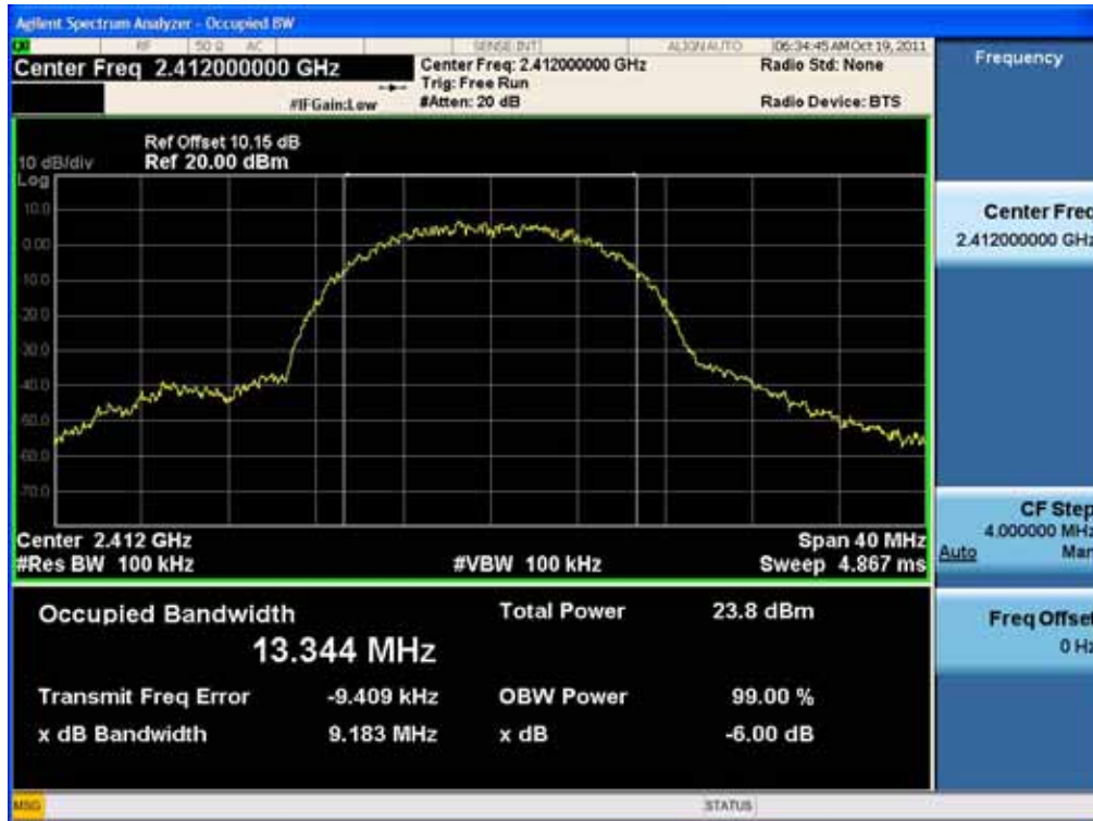
6dB Bandwidth plot (802.11b-CH 1)
