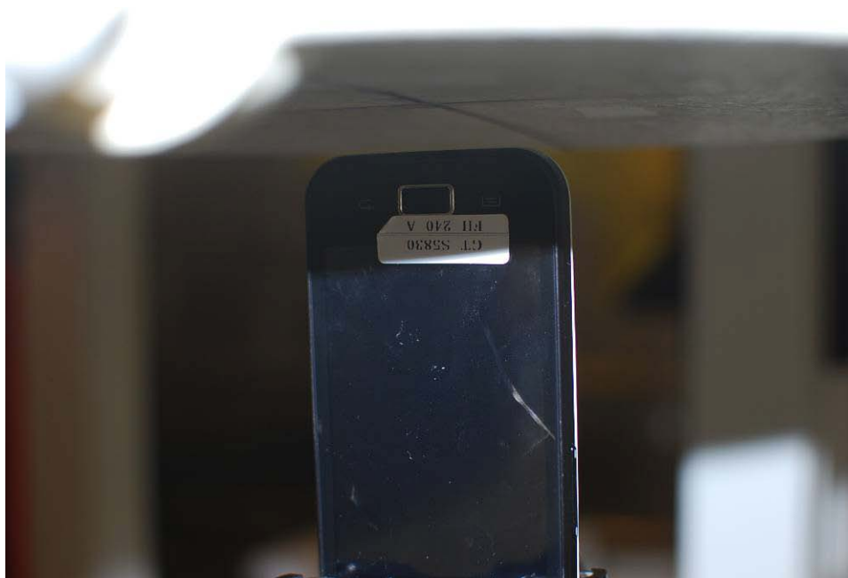
Figure 21-10 SAR Test Setup Photo 10 – Edge C at 1.0 cm
