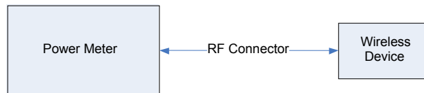
Figure 12-1 Power Measurement Setup
