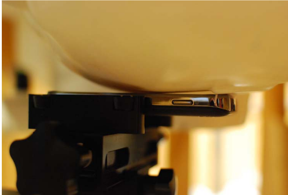
Figure 21-3 SAR Test Setup Photo 3: Left Touch
