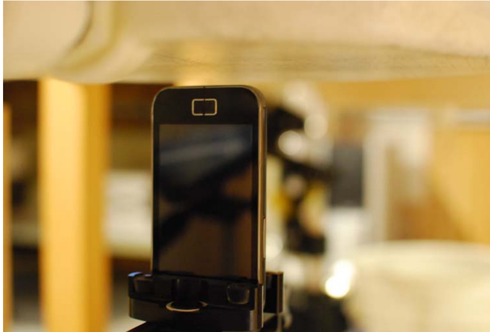
Figure 21-9 SAR Test Setup Photo 9: Bottom at 1.0 cm
