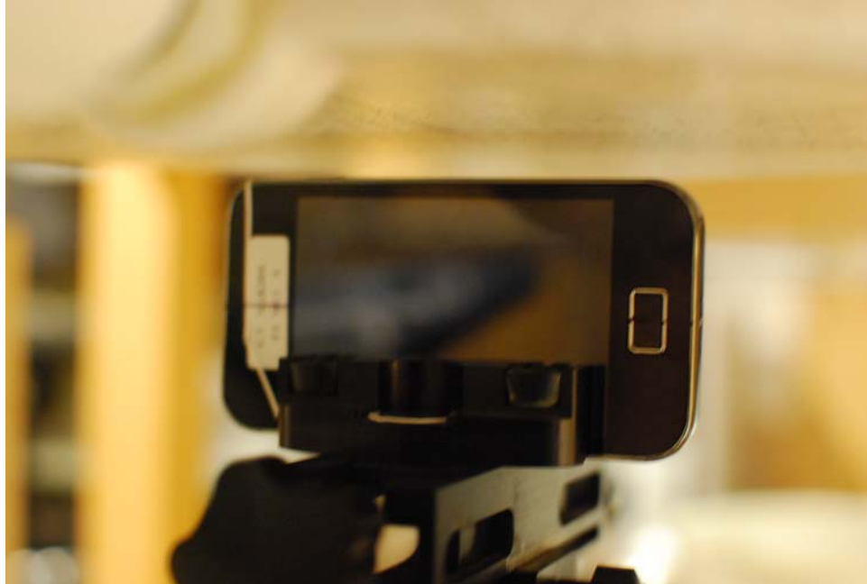
Figure 21-7 SAR Test Setup Photo 7: Right at 1.0 cm
