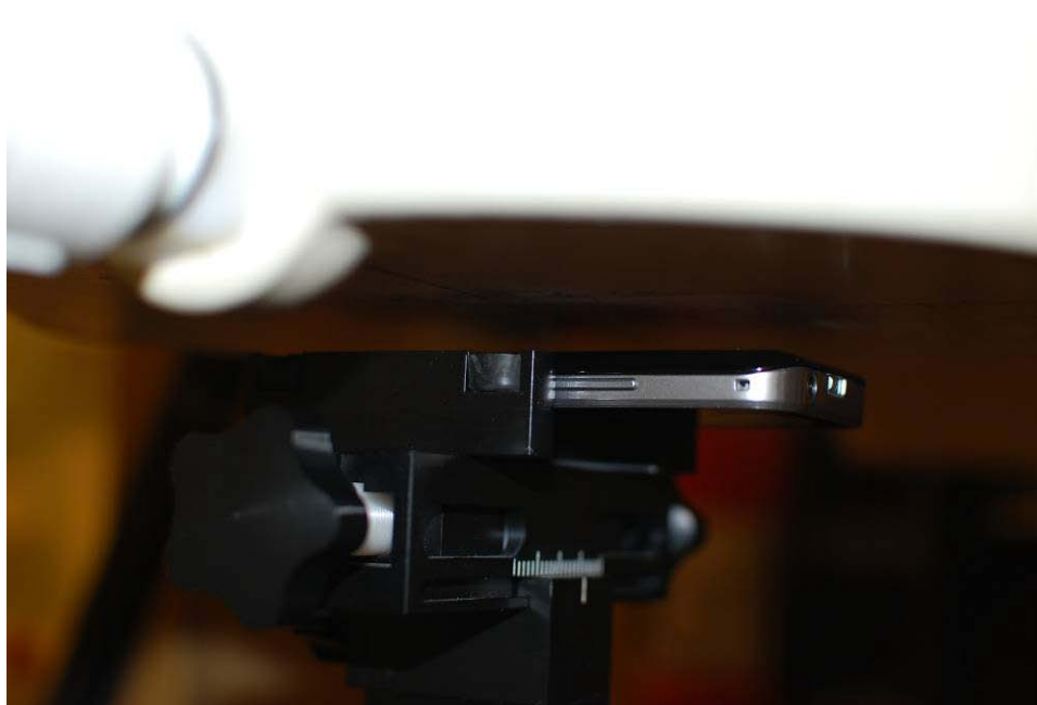
Figure 21-5 SAR Test Setup Photo – Back at 1.0 cm
