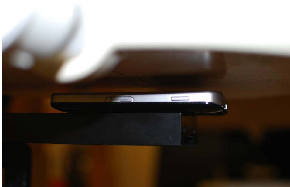
Figure 21-6 SAR Test Setup Photo – Front at 1.0 cm
