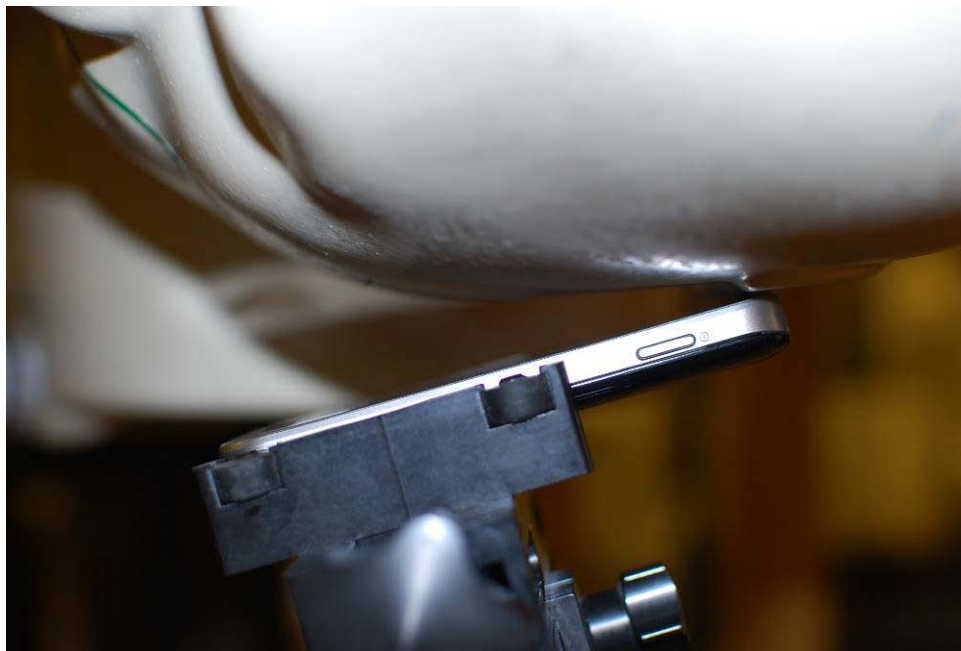
Figure 21-4 SAR Test Setup Photo – Left Tilt
