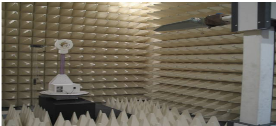
Figure2. Photograph of 3m Fully-Anechoic Chamber
