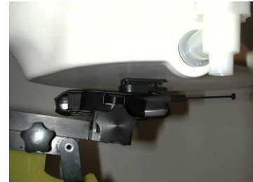
Figure 8-4 Body SAR Sample Photo (Not Actual EUT)
