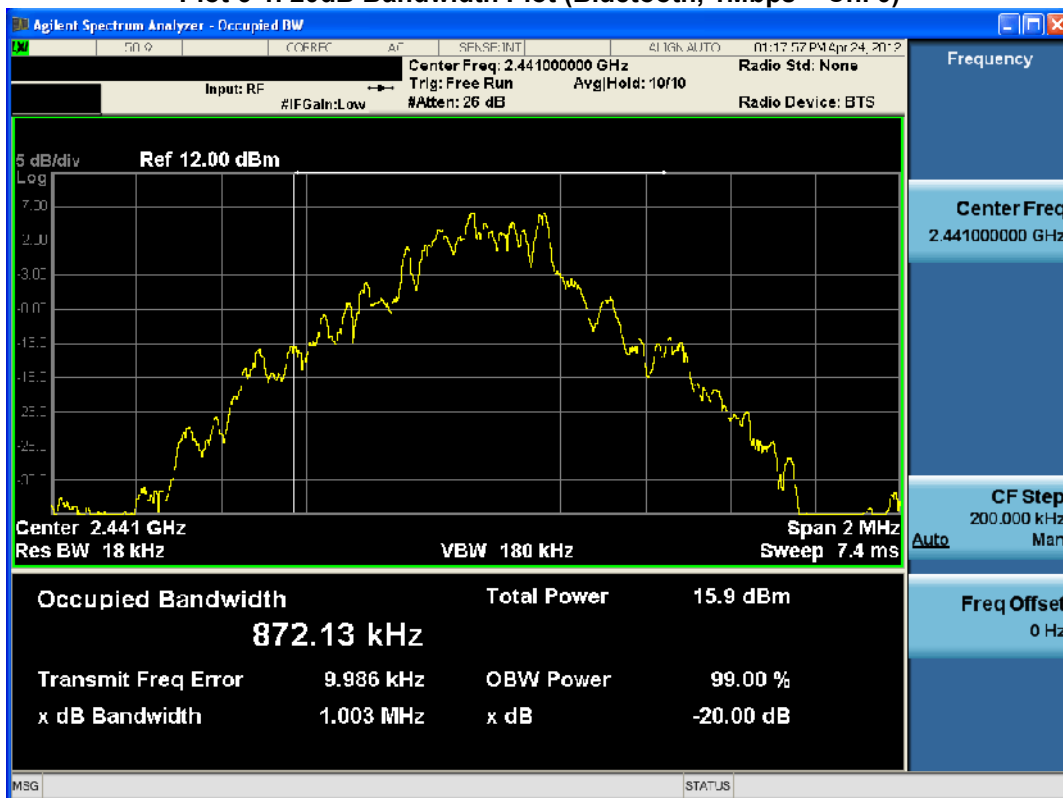
Plot 6-2. 20dB Bandwidth Plot (Bluetooth, 1Mbps – Ch. 39)
