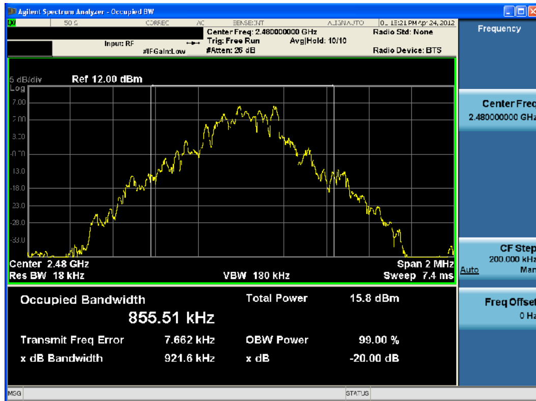
Plot 6-3. 20dB Bandwidth Plot (Bluetooth, 1Mbps – Ch. 78)
