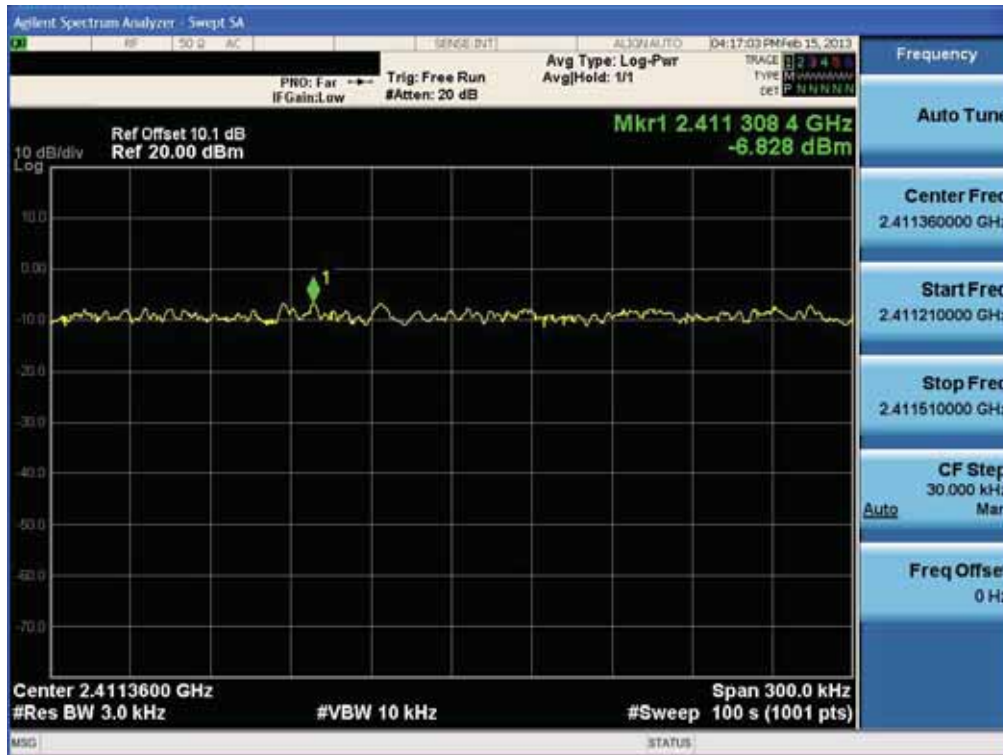
Power Spectral Density (802.11b-CH 6)
