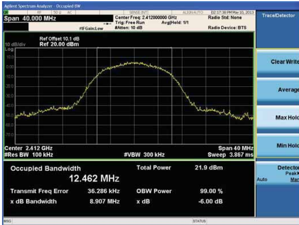
6dB Bandwidth plot (802.11b-CH 6)
