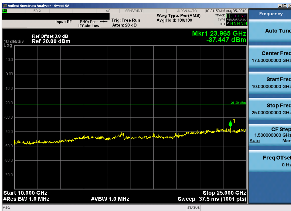
Plot 6-14. Conducted Spurious Plot (802.11b – Ch. 1)
