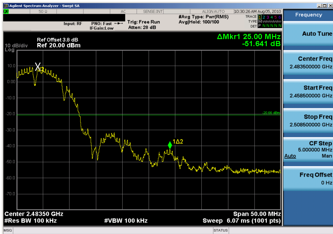
Plot 6-8. Band Edge Plot (802.11b – Ch. 11)
