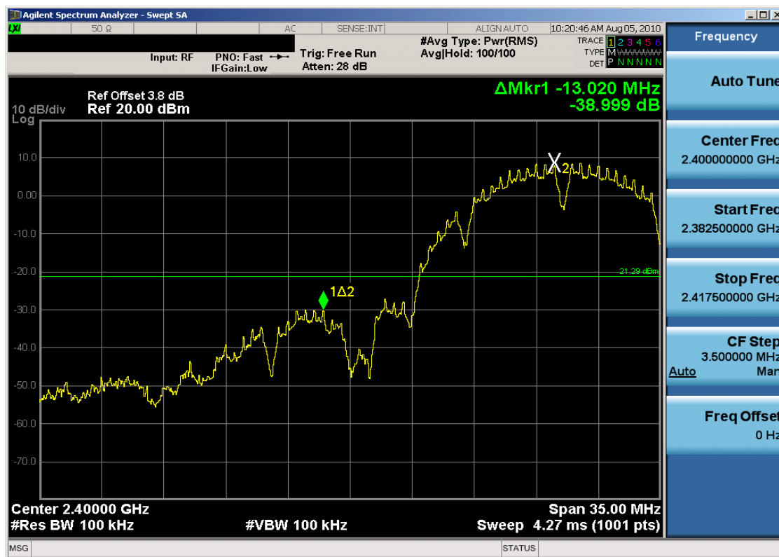
Plot 6-7. Band Edge Plot (802.11b – Ch. 1)
