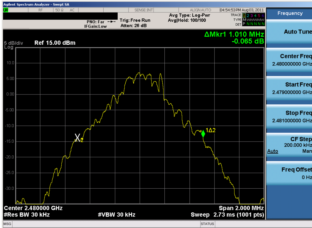
Plot 6-3. 20dB Bandwidth Plot (Bluetooth, 1Mbps – Ch. 78)
