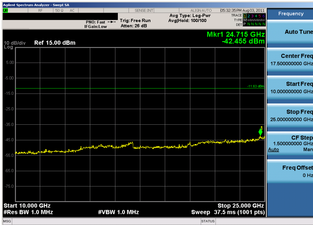
Plot 6-21. Conducted Spurious Plot (Bluetooth, 1Mbps – Ch. 39)
