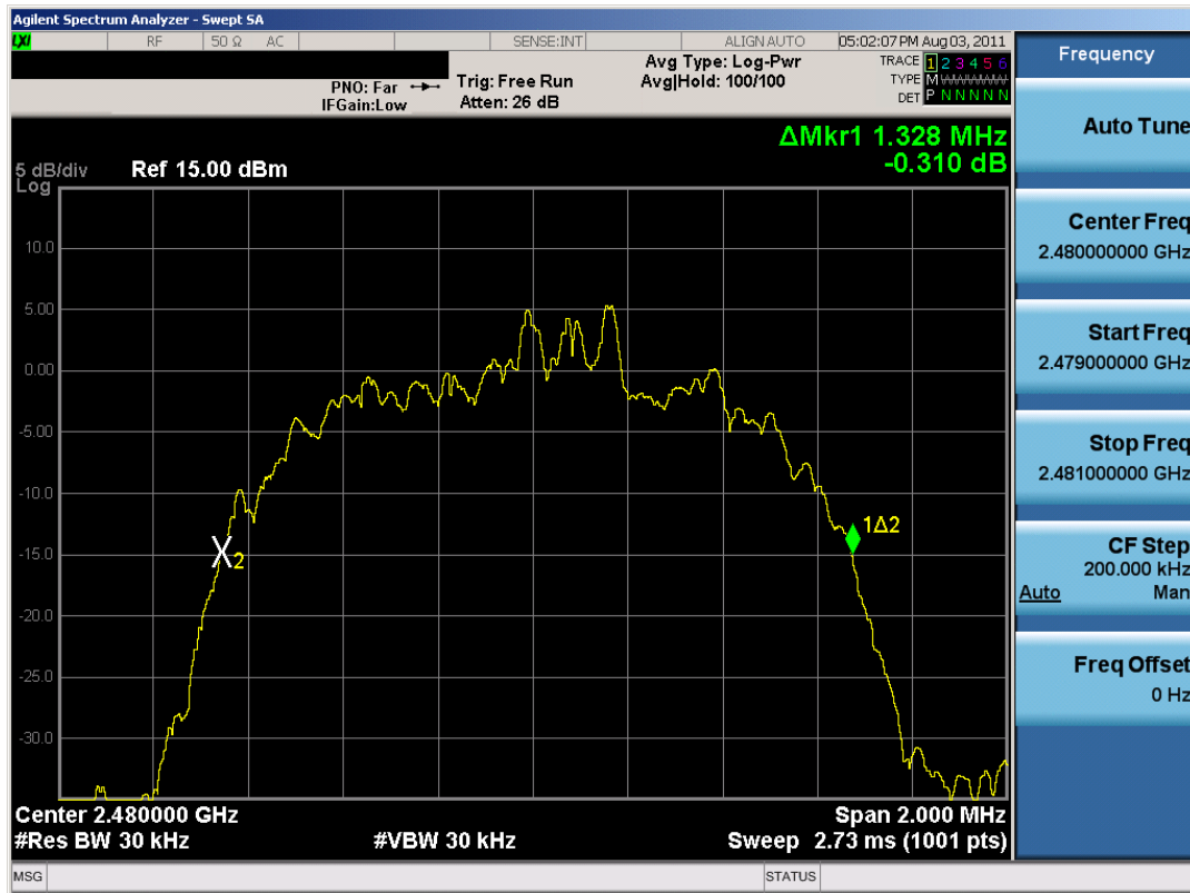
Plot 6-9. 20dB Bandwidth Plot (Bluetooth, 3Mbps – Ch. 78)
