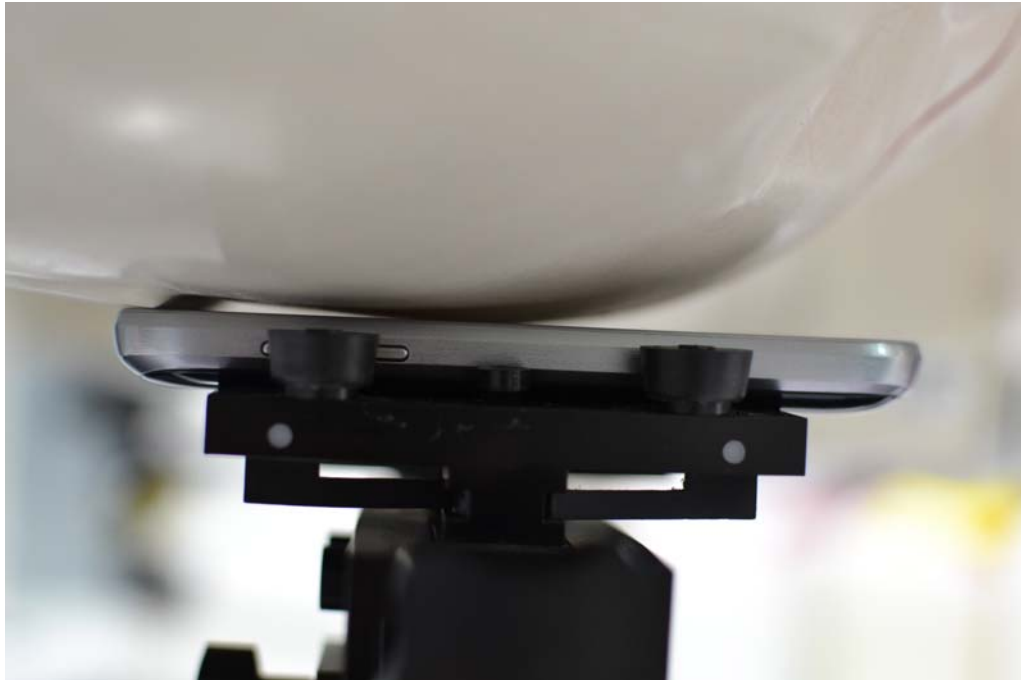
SAR Test Setup Photo 1 – Right Cheek
