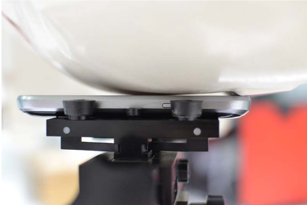
SAR Test Setup Photo 3 – Left Cheek
