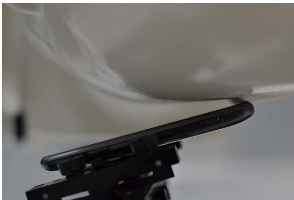
SAR Test Setup Photo 4 – Left Tilt
