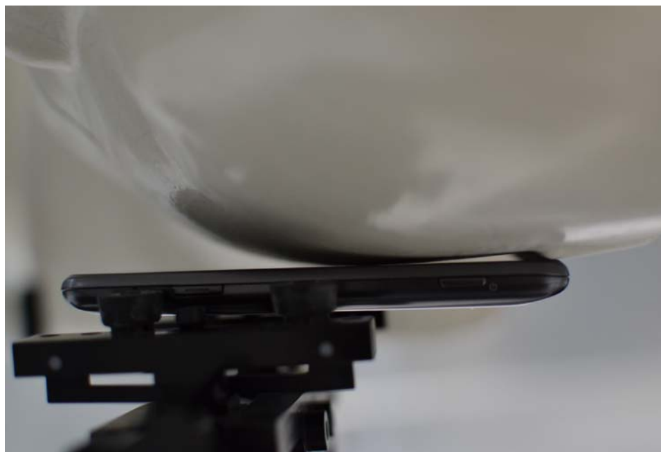
SAR Test Setup Photo 3 – Left Touch
