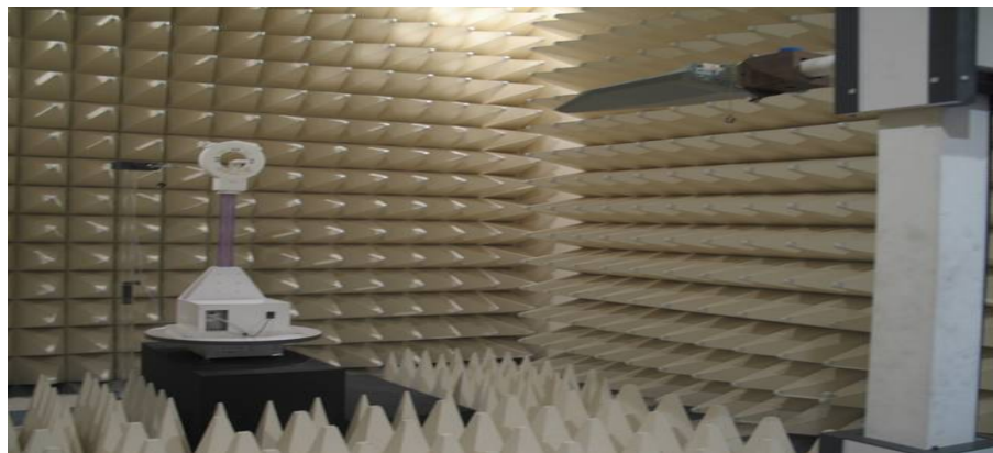
Figure2. Photograph of 3m Fully-Anechoic Chamber
