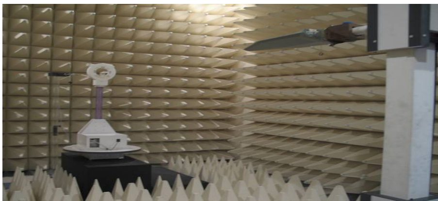
Figure2. Photograph of 3m Fully-Anechoic Chamber
