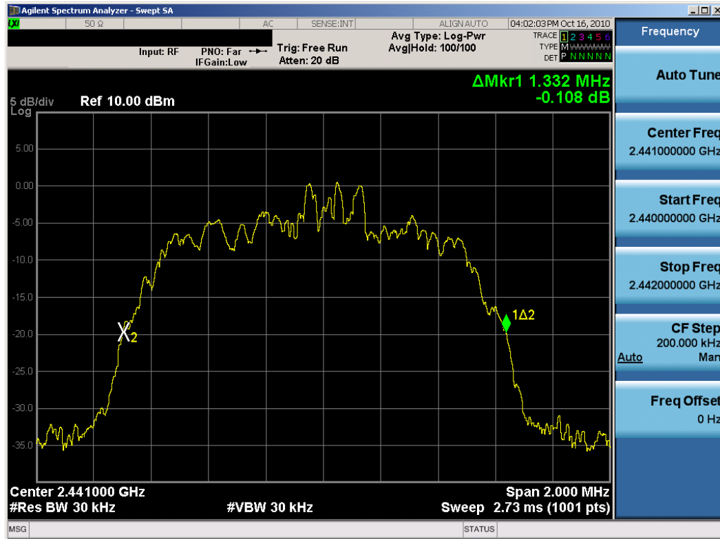
Plot 6-2. 20dB Bandwidth Plot (Bluetooth (EDR) – Ch. 39)
