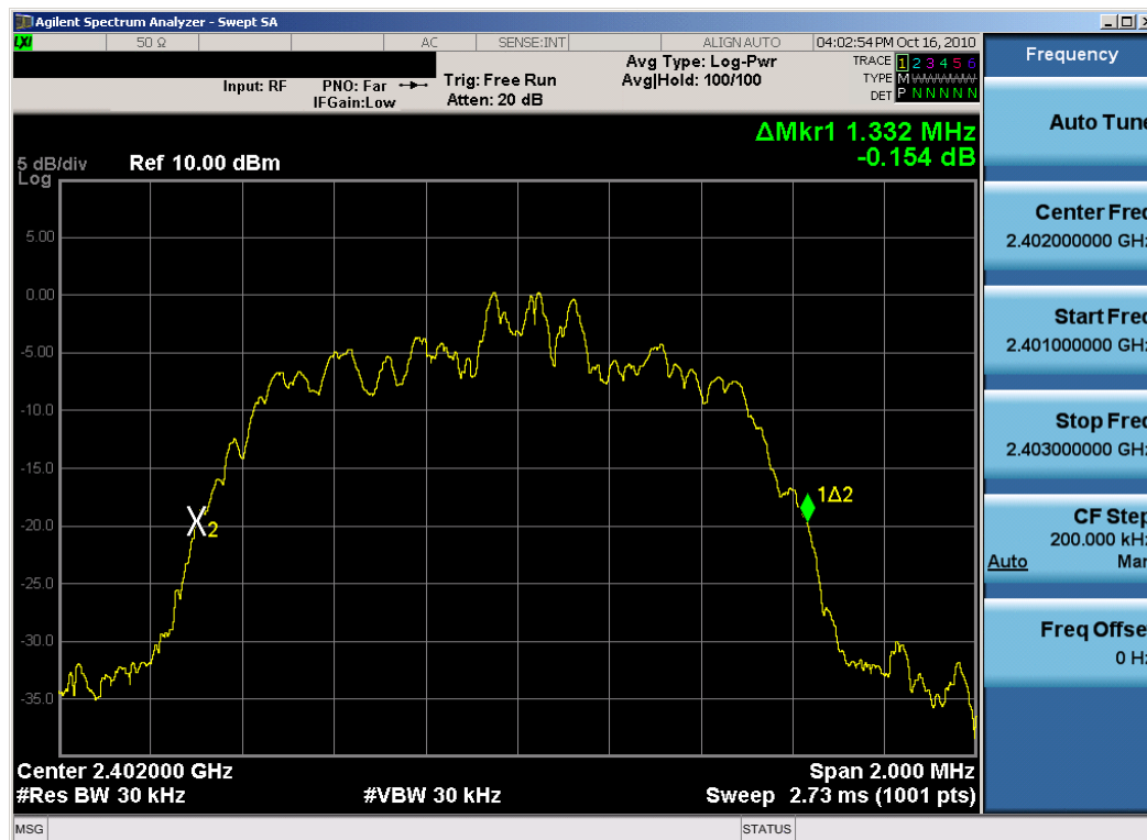
Plot 6-1. 20dB Bandwidth Plot (Bluetooth (EDR) – Ch. 0)
