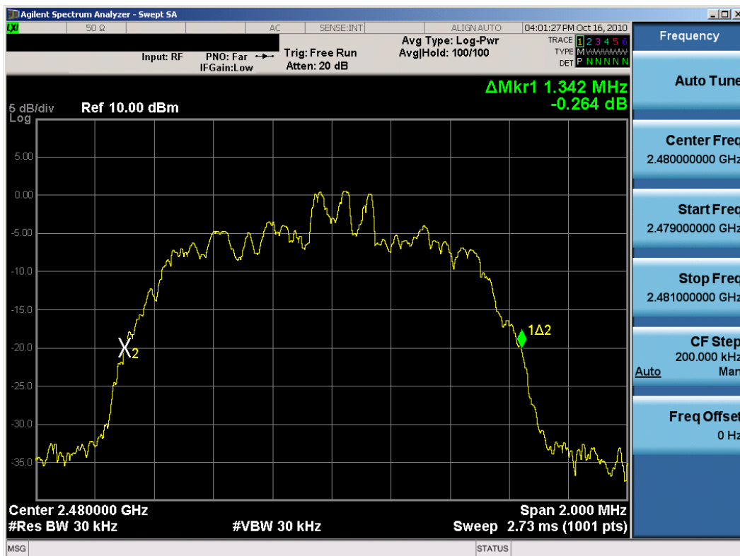
Plot 6-3. 20dB Bandwidth Plot (Bluetooth (EDR) – Ch. 78)
