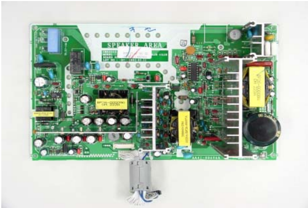
POWER BOARD TOP VIEW
