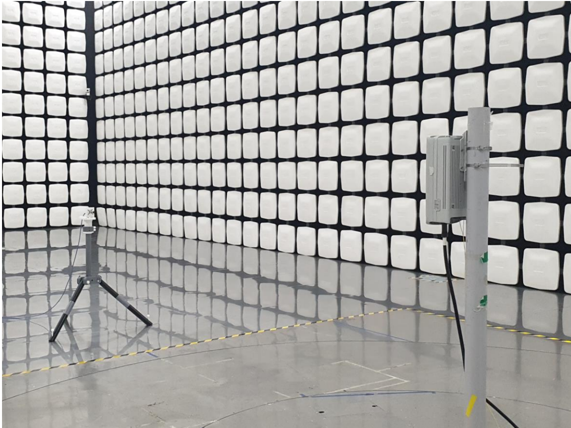
Radiated Test Setup Photo – Spurious (90 GHz ~ 140 GHz)
