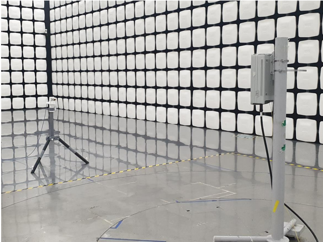
Radiated Test Setup Photo – Spurious (60 GHz ~ 90 GHz)
