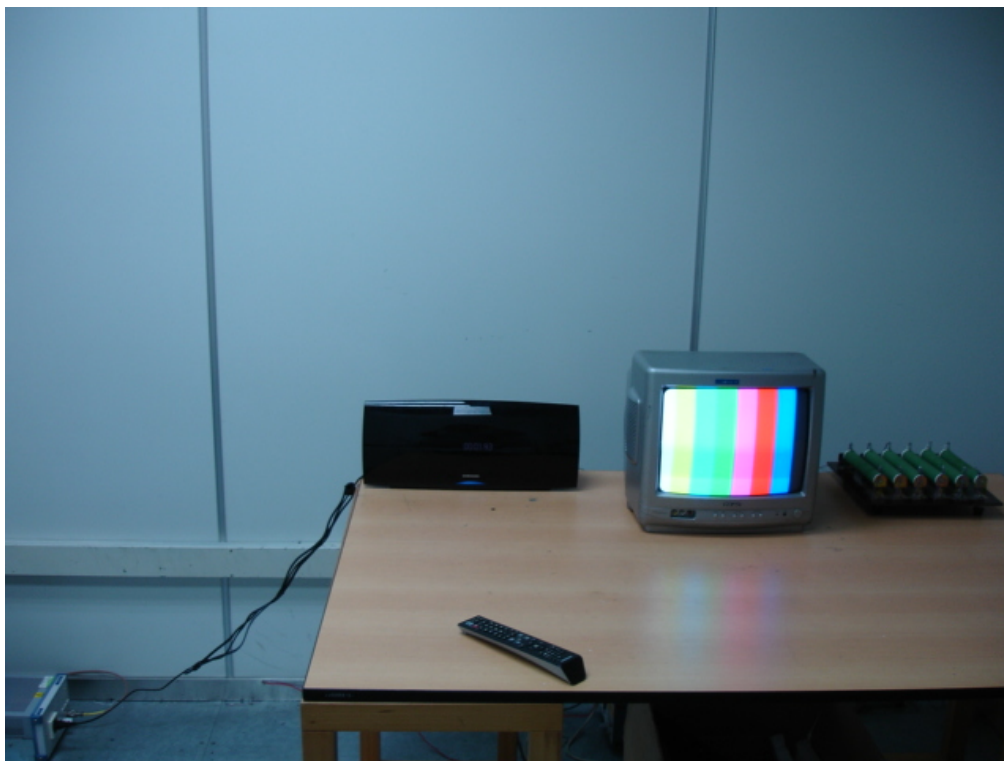
Photo 2 Antenna Terminal Voltage Disturbance Test
