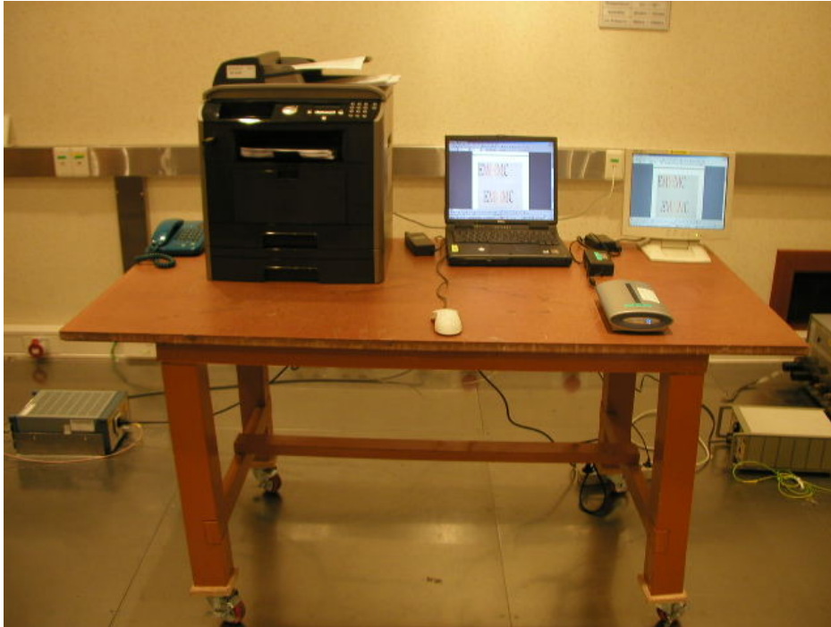
Pic. 1 Conducted Emission (Front)
