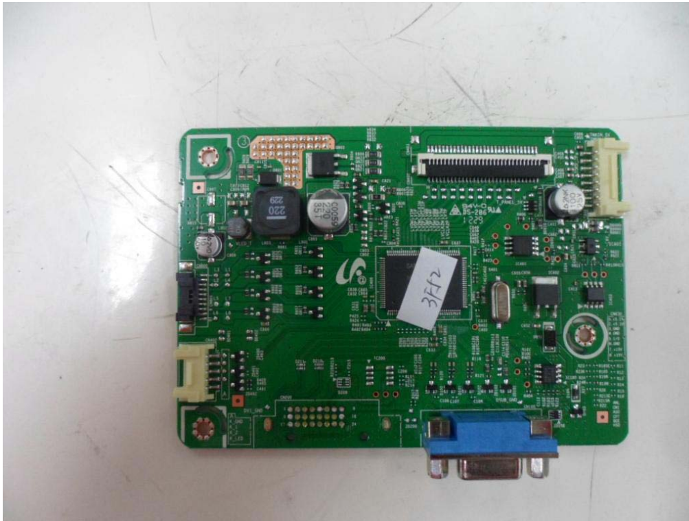
Before change BN41-01916A(old) internal front view
