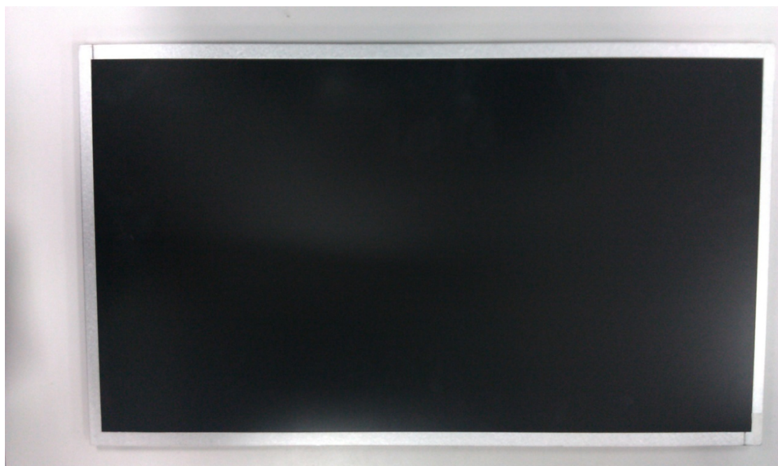
After change M185BGE-L22 Internal front view
