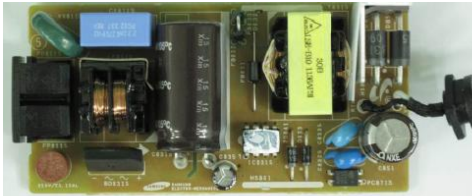
Before change AD-3014B internal front view
