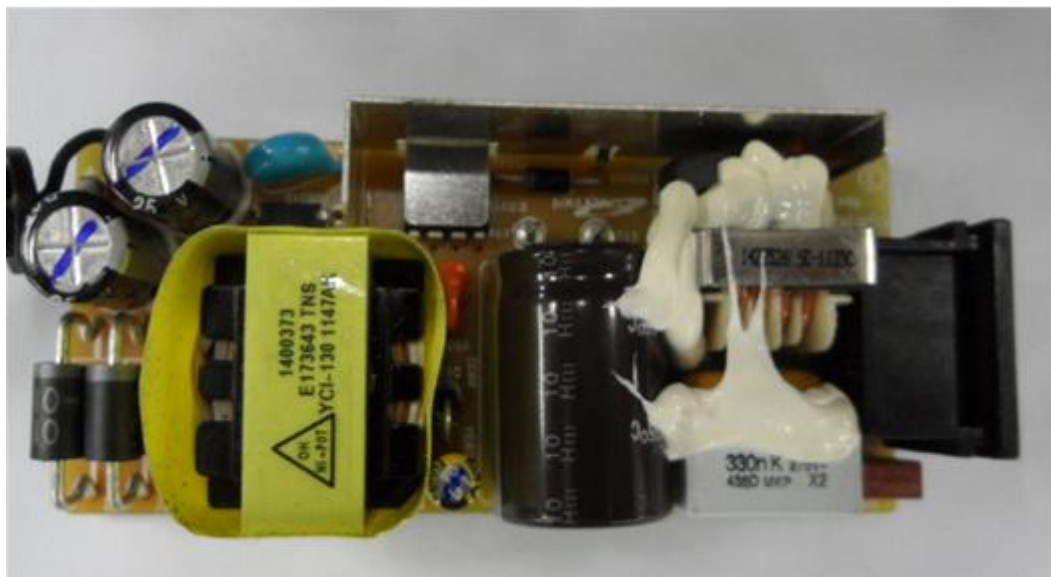
Back change PS30W-14J1 internal front view
